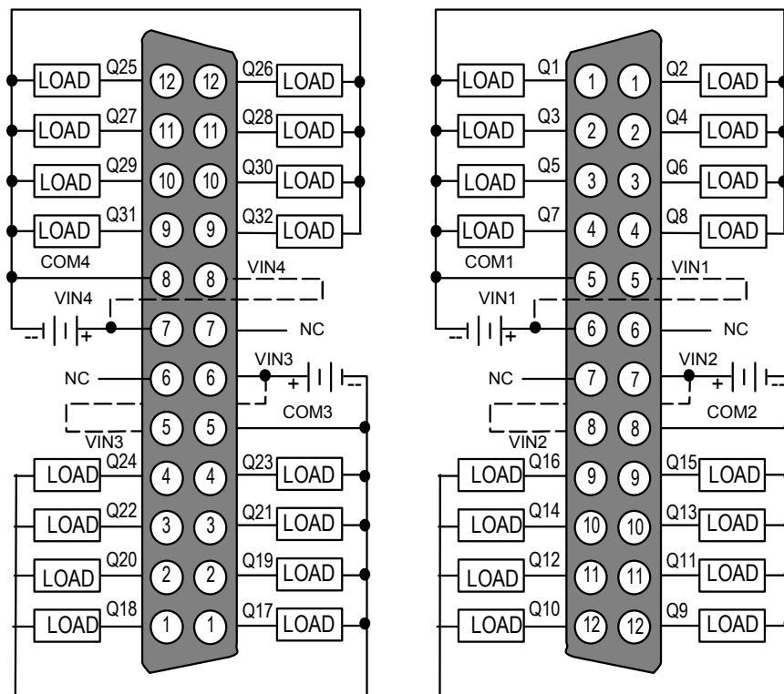
If the total current is greater than 3 Amps for a group, use both  $V_{IN}$  pins for the group by adding a second wire (shown by dashed lines above).
