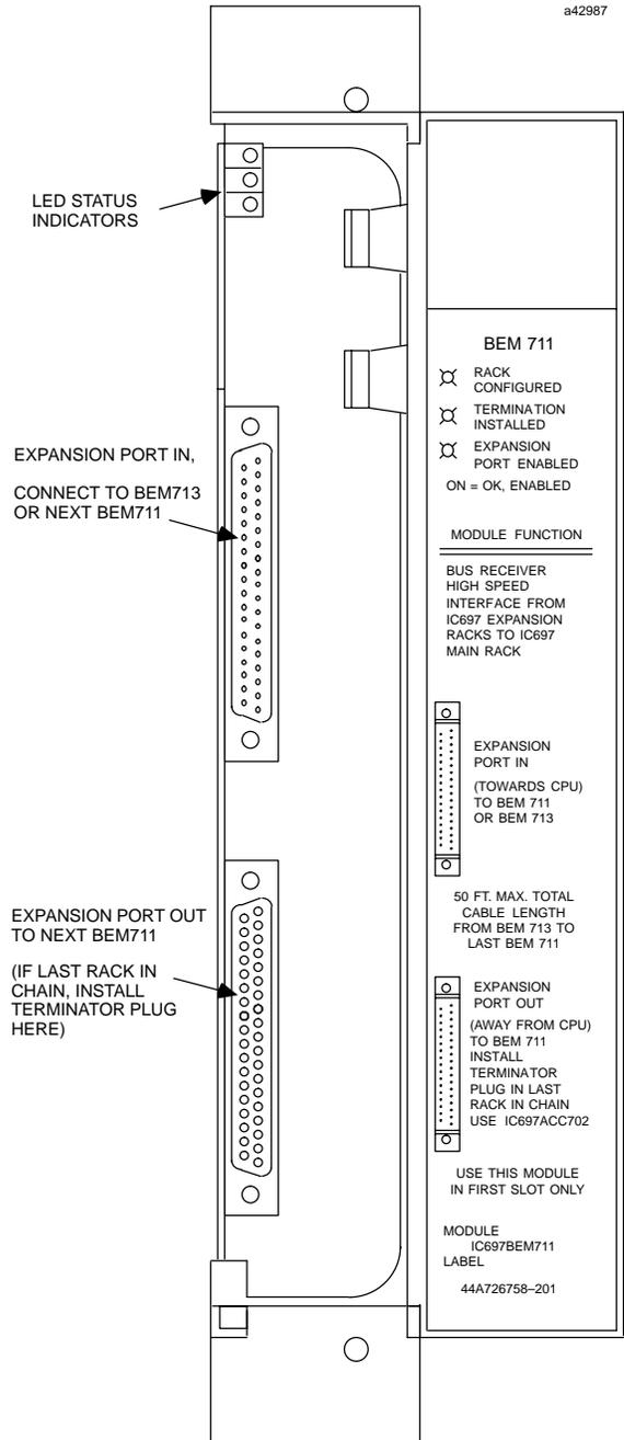
Figure 3. Bus Receiver Module - User Details
