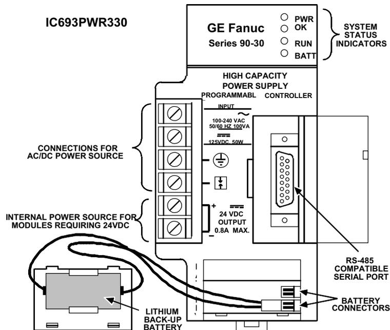
**Figure 4-2. High Capacity AC/DC Input Power Supply - IC693PWR330**
