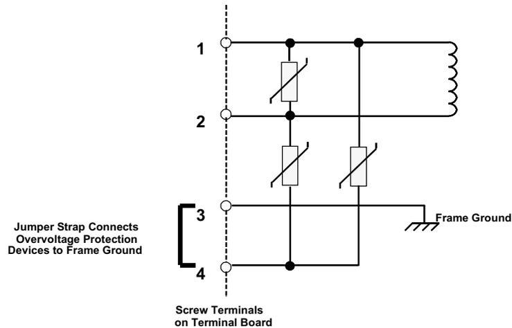
Figure 4-3. Overvoltage Protection Devices and Jumper Strap
