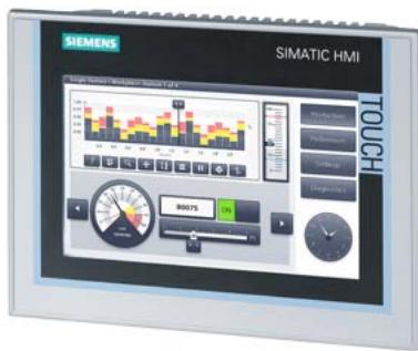
SIMATIC HMI TP700 Comfort, Comfort Panel, touch operation, 7" widescreen TFT display, 16 million colors, PROFINET interface, MPI/PROFIBUS DP interface, 12 MB configuration memory, Windows CE 6.0, configurable from WinCC Comfort V11
