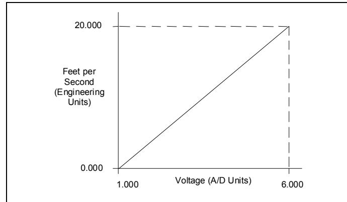
For this example, 1.0V to 6.0V is the normal voltage range, but the module will attempt to scale the inputs for a voltage that lies outside the range. If a voltage of 10.0V were input to the channel, the module would return a scaled channel value of 36.000. The application should use alarms or take other precautions for scaled inputs that are outside the acceptable range or invalid.
