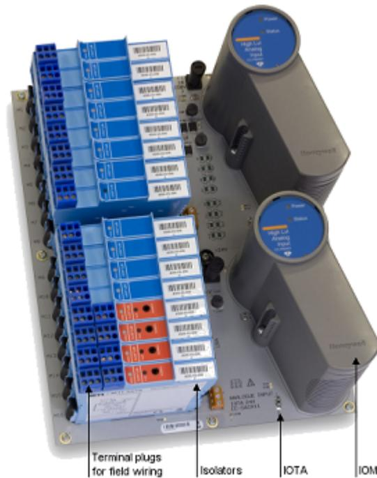
Figure 237: GI/IS board assembly
