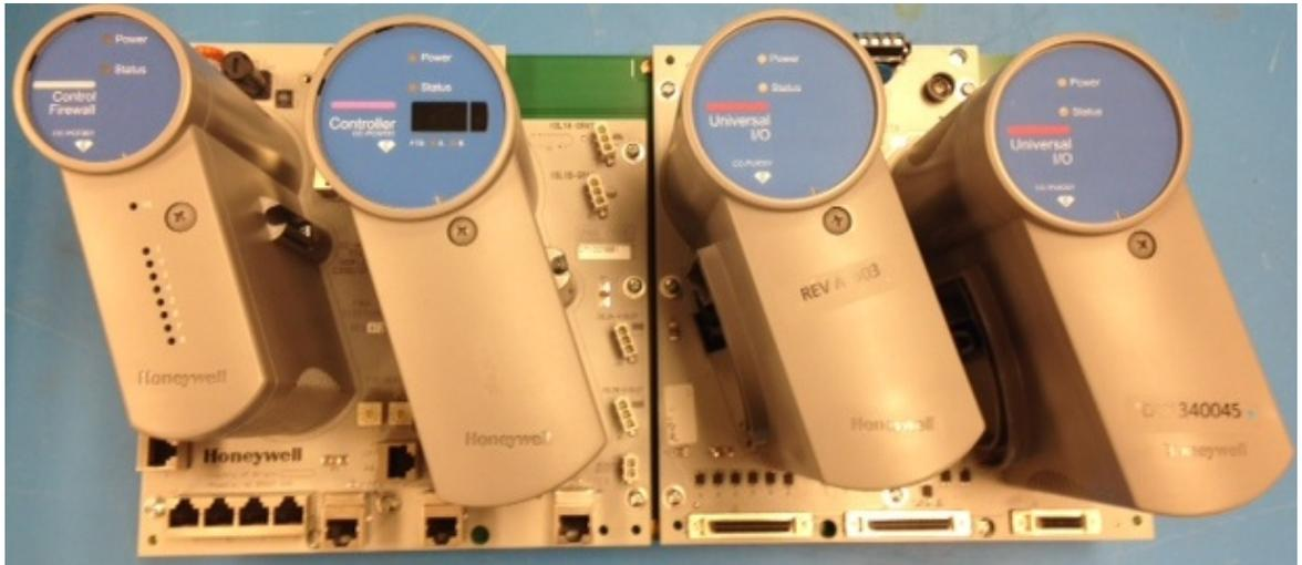
Figure 2: View of Universal Horizontal Input/Output (UHIO)
