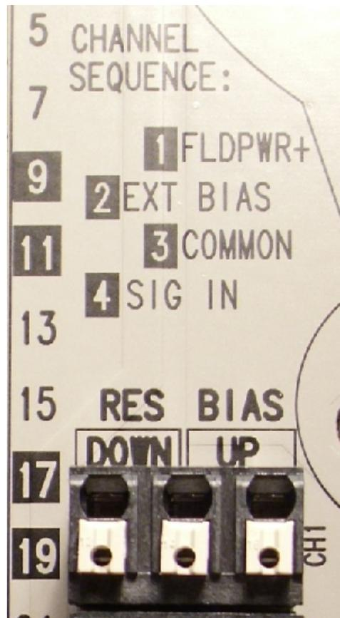
Figure 101: RES BIAS Terminal Block (channel 1 shown)
