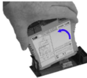
Figure 268: Removing a module from an IOTA
