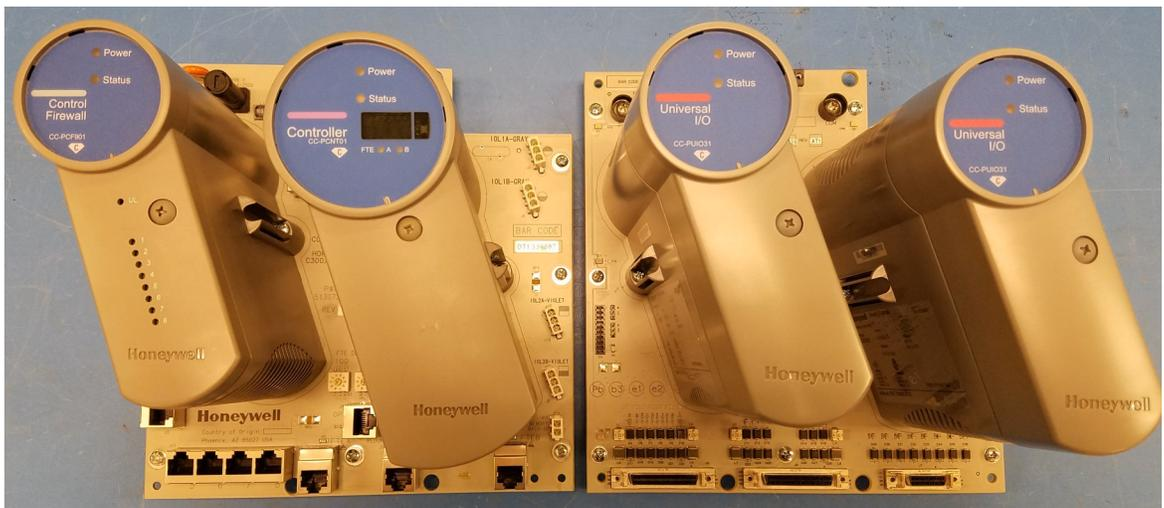
Figure 3: View of Universal Horizontal Input/Output Two (UHIO-2)
