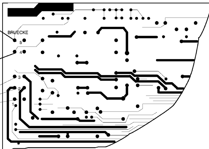
Figure 17.15 Locations of Jumpers for Setting Rated Nominal Current of Current Inputs (Production Series /JH or Earlier).
