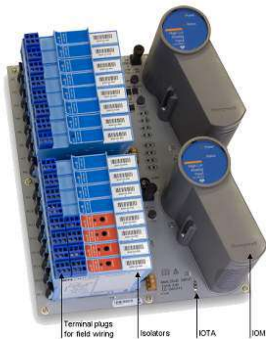
Figure 237: GI/IS board assembly
