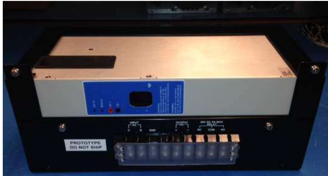
Figure 133: UHIO Power supply
