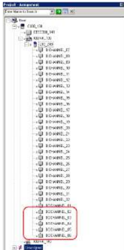
Figure 186: Appearance of DO channels before ganging
