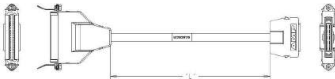
Figure 138: UHIO cable adapter
