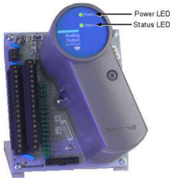
Figure 214: Series C I/O LED indicators
