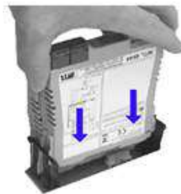
Figure 239: Mounting a module onto an IOTA
