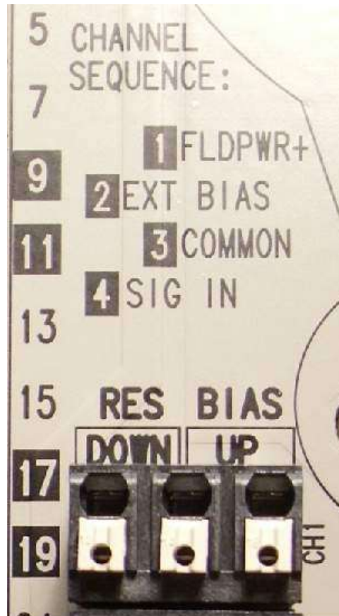
Figure 101: RES BIAS Terminal Block (channel 1 shown)
