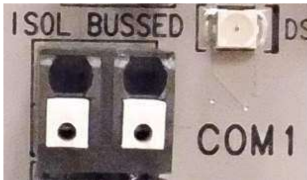
Figure 105: ISOL/BUSSED terminal blocks
