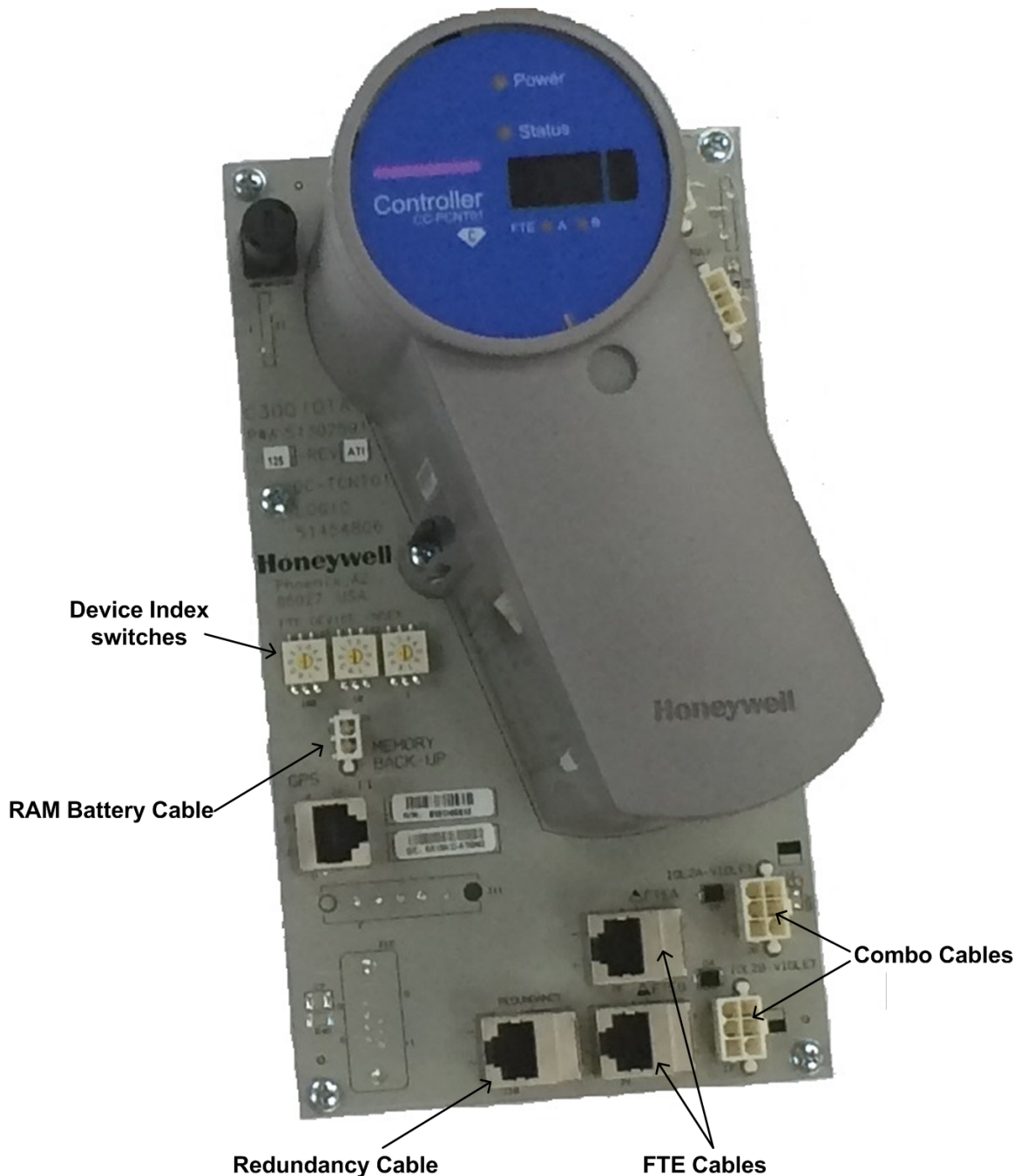
Figure 4.4 C300 Controller IOTA Board Features
