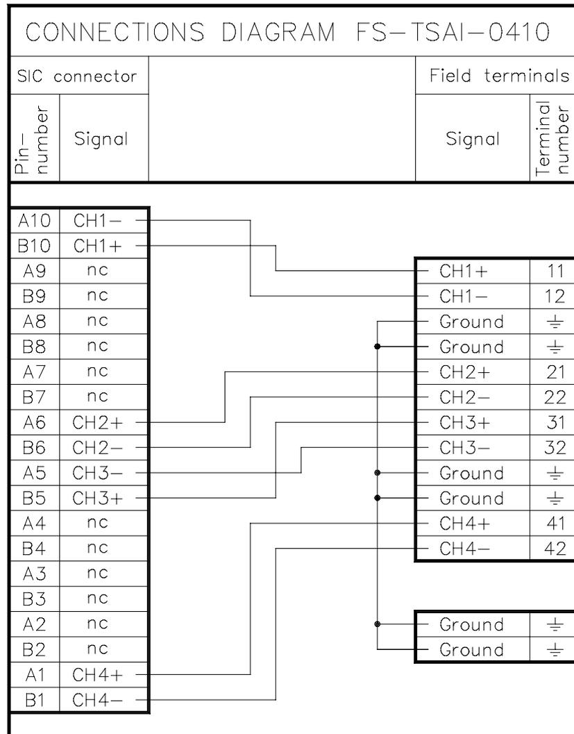
Figure 2 Connections diagram
