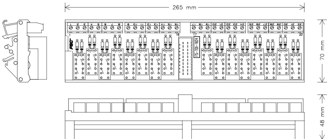
Figure 1 Mechanical layout
