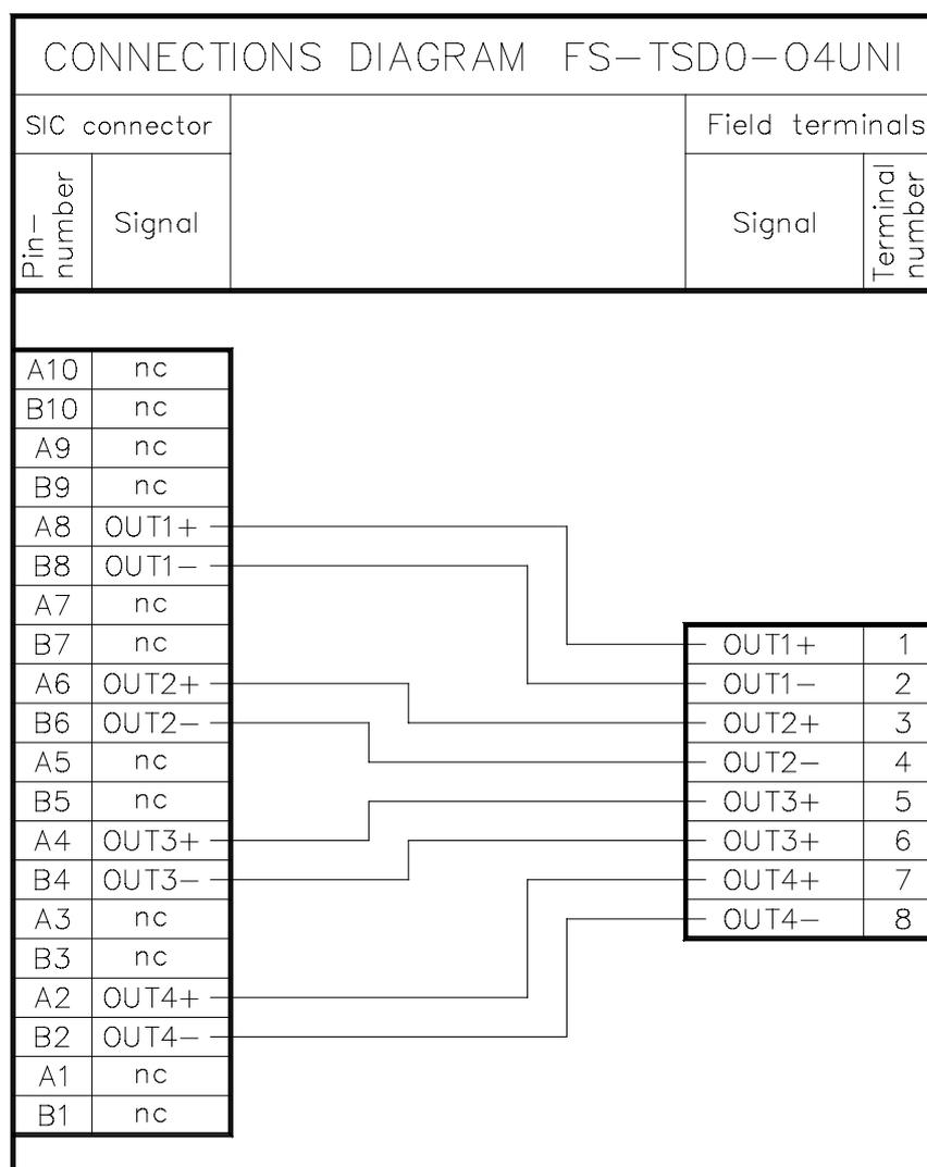
Figure 2 Connections diagram
