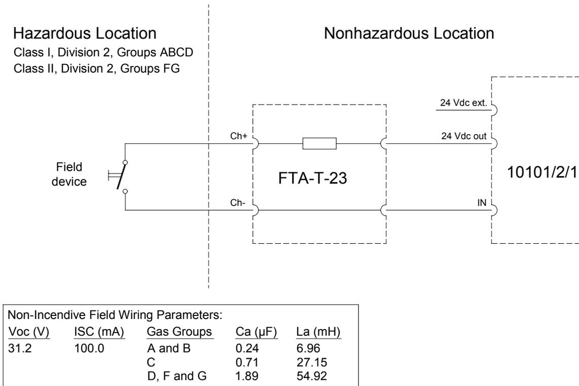
Figure 5 Connection of input in hazardous locations
