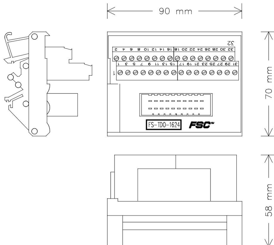
Figure 1 Mechanical layout
