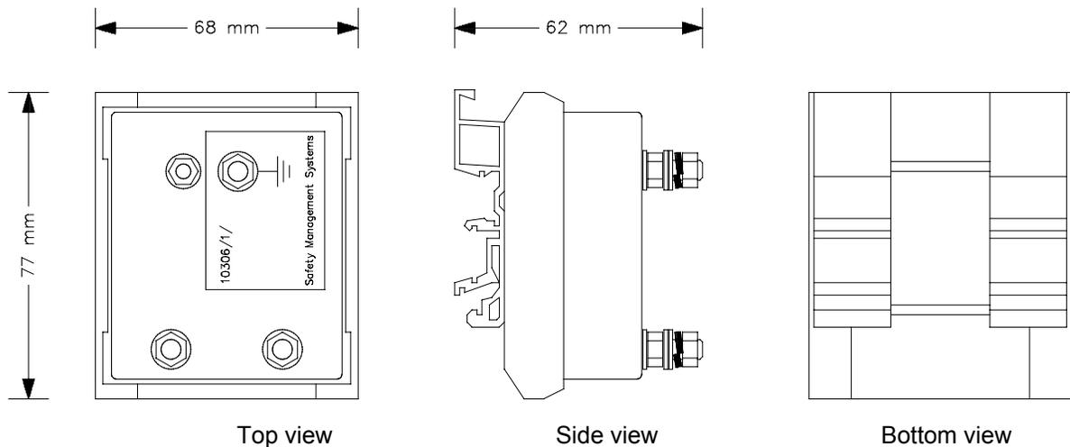
Figure 1 10306/1/. mechanical layout
