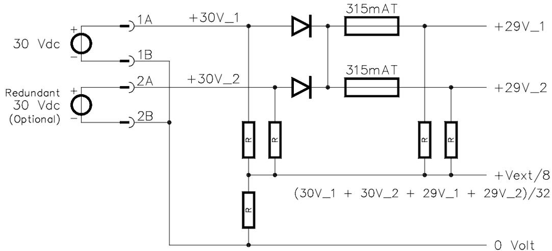
Figure 4 Schematic diagram for power distribution with monitoring
