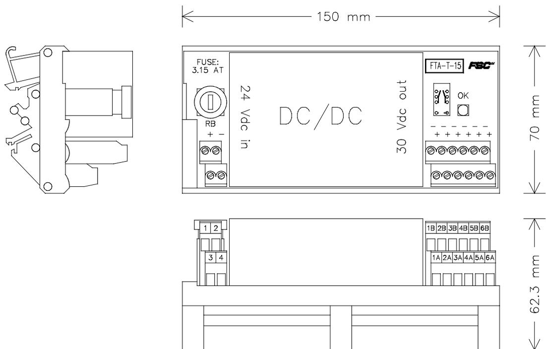
Figure 1 Mechanical layout
