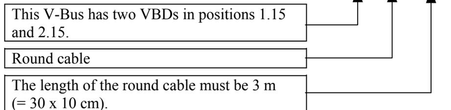
As the distance between the CP1 connector and the CP2 connector is 20 cm (7.9 in), the round cable will have a total length of approx. 320 cm (10.5 ft).
