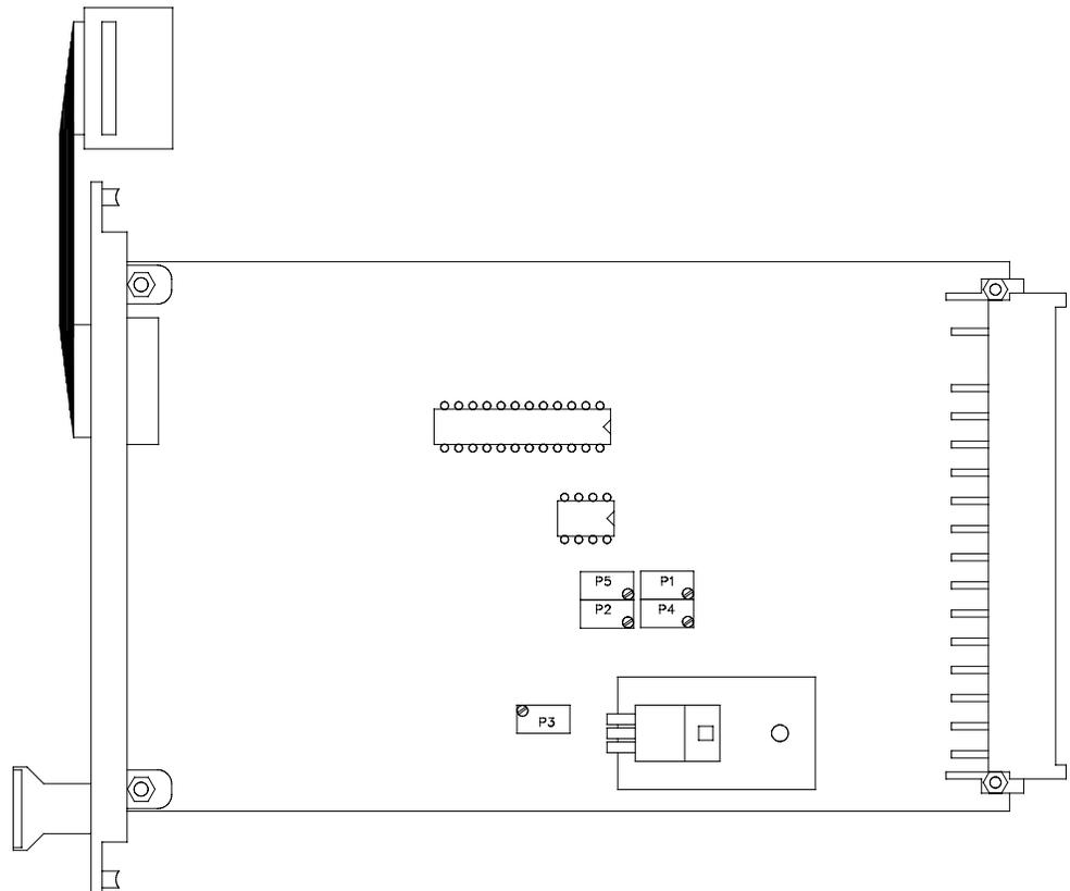
Figure 4 Location of potentiometers on 10102/2/1 module
