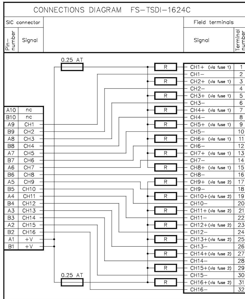
Figure 2 Connections diagram
