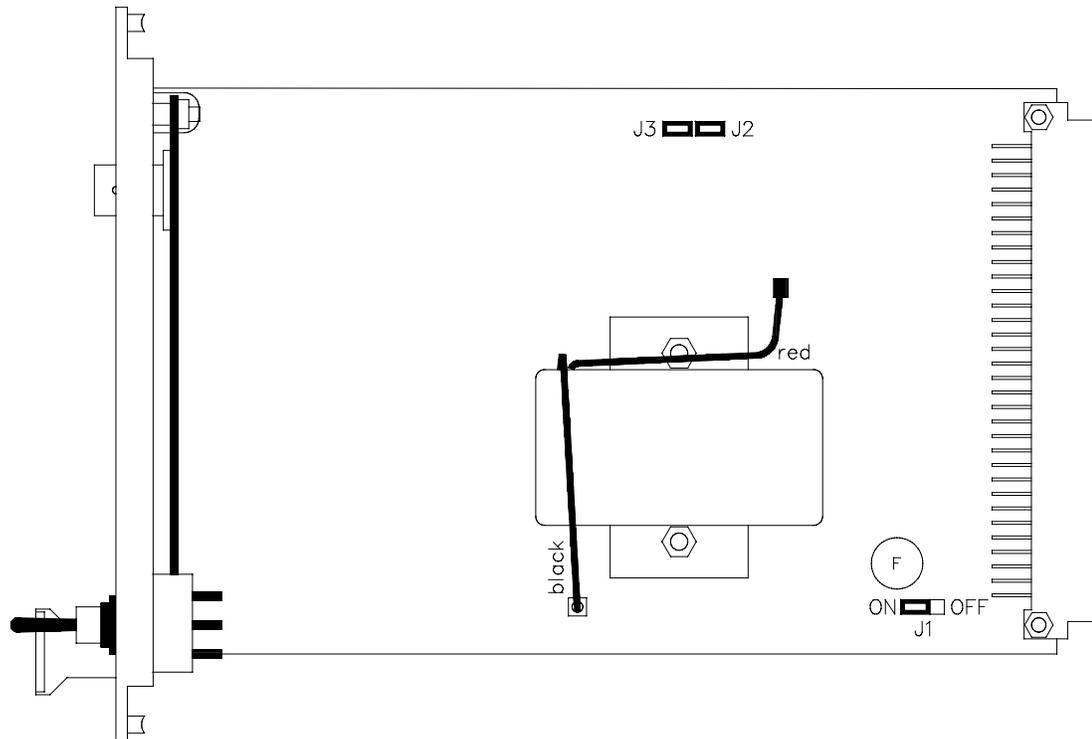
Figure 2 Jumper settings on 10006/2/2 module (08905 shown)
