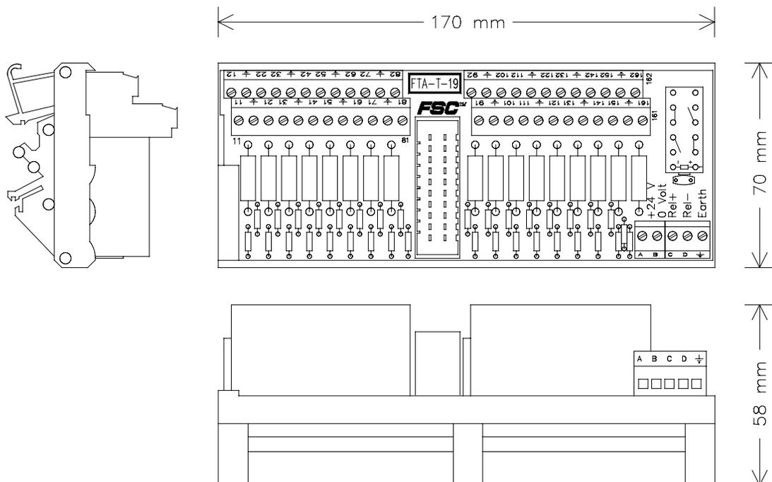
Figure 1 Mechanical layout
