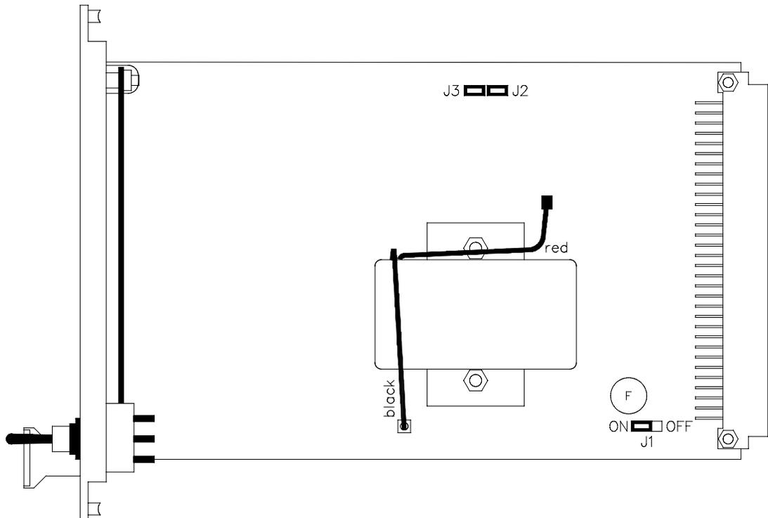
Figure 2 Jumper settings on 10006/2/1 module (08804 shown)
