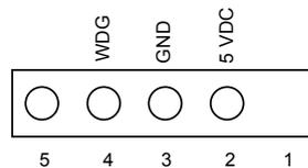
Figure 4 Connector CN22 (detail)
