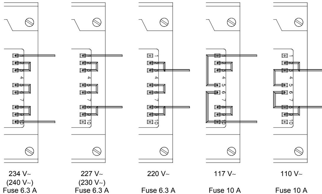
Figure 4 Transformer connections
