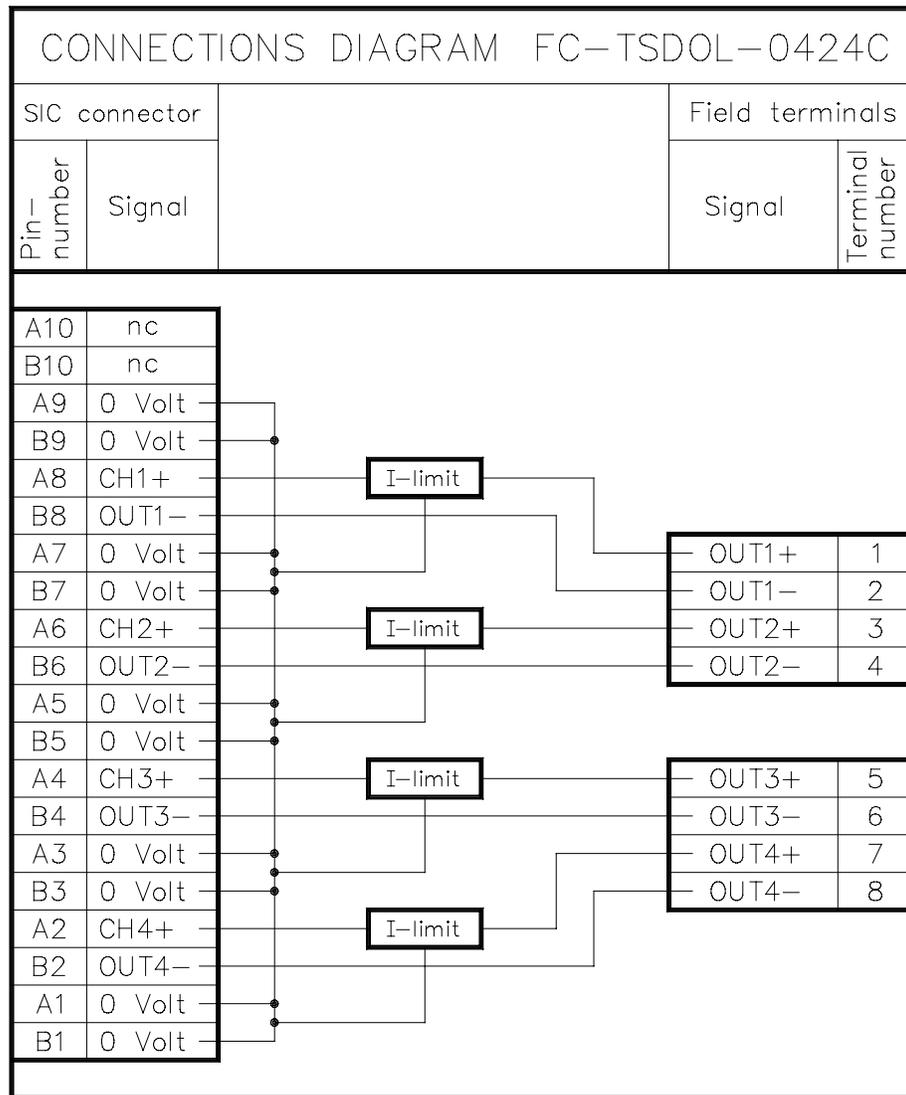
Figure 3 Connections diagram
