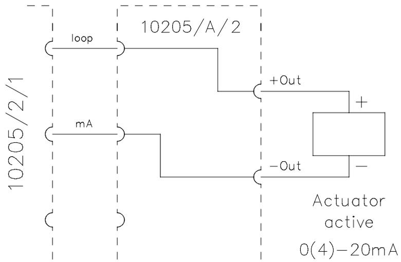
Figure 3 Schematic diagram of a 10205/A/2 module
