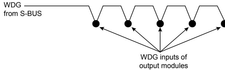
Figure 3 Watchdog wiring
