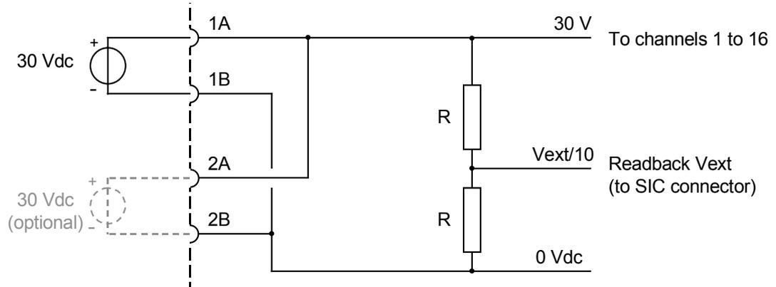
Figure 3 Schematic diagram for power distribution with monitoring
