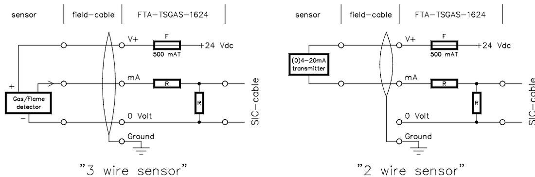
Figure 2 Schematic diagram for connecting a transmitter
