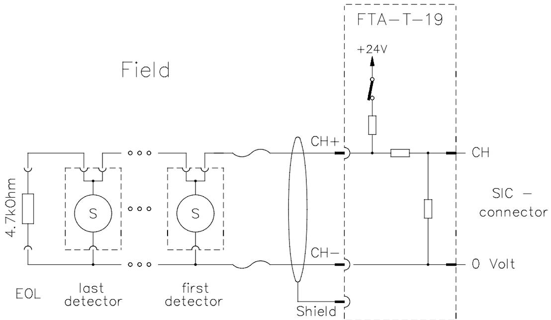
Figure 2 Typical schematic diagram for FTA-T-19 input
