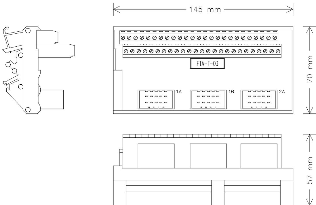
Figure 1 Mechanical layout
