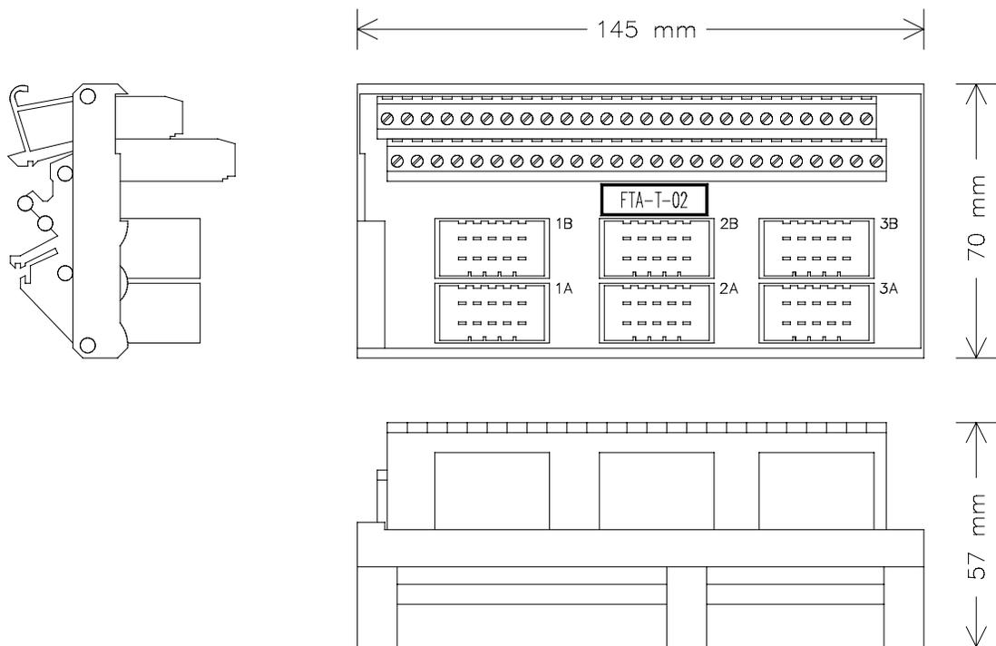
Figure 1 Mechanical layout
