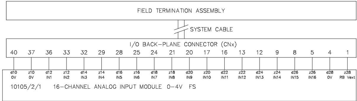
Figure 2 Connection example of 10105/2/1 module to FTA
