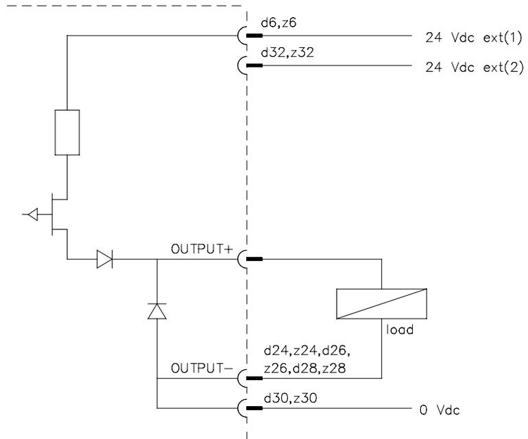
Figure 1 Schematic diagram for connection of one output to the 10206/2/1 module
