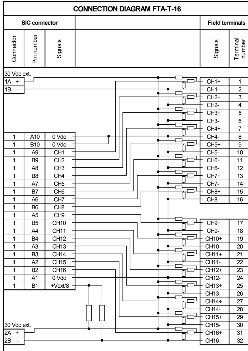
Figure 4 Connections diagram
