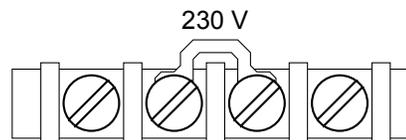
Figure 6 Selector block set at 230 V
