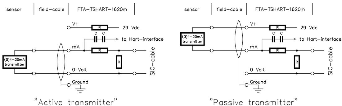
Figure 2 Schematic diagram for connecting a transmitter
