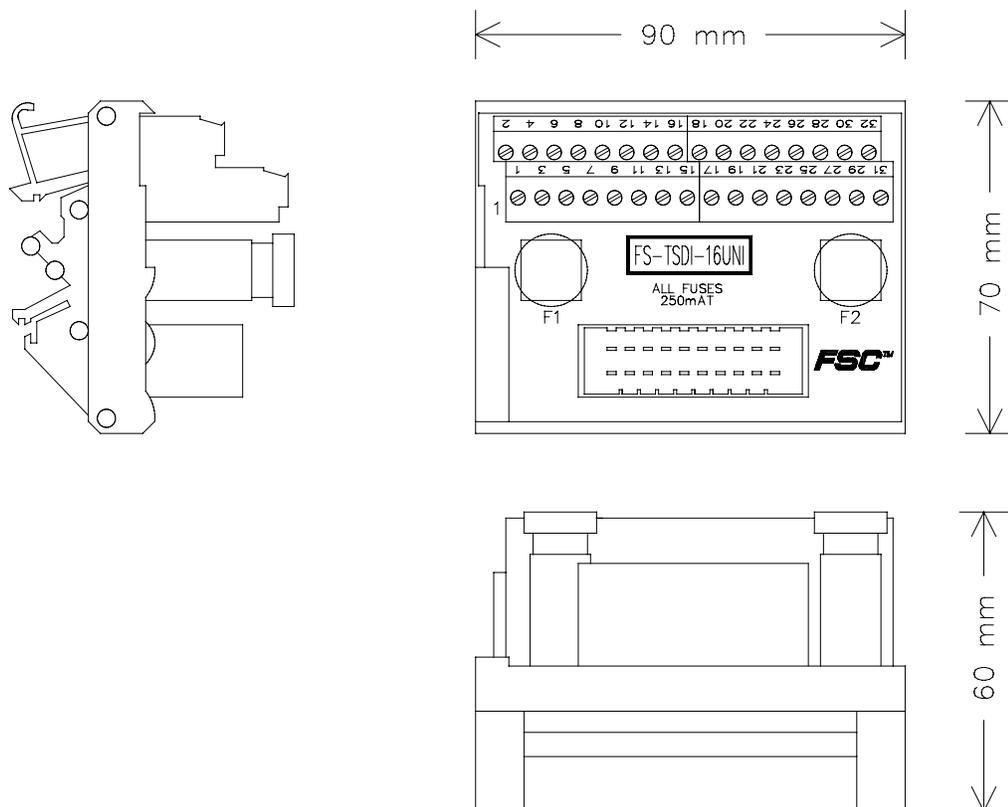
Figure 1 Mechanical layout
