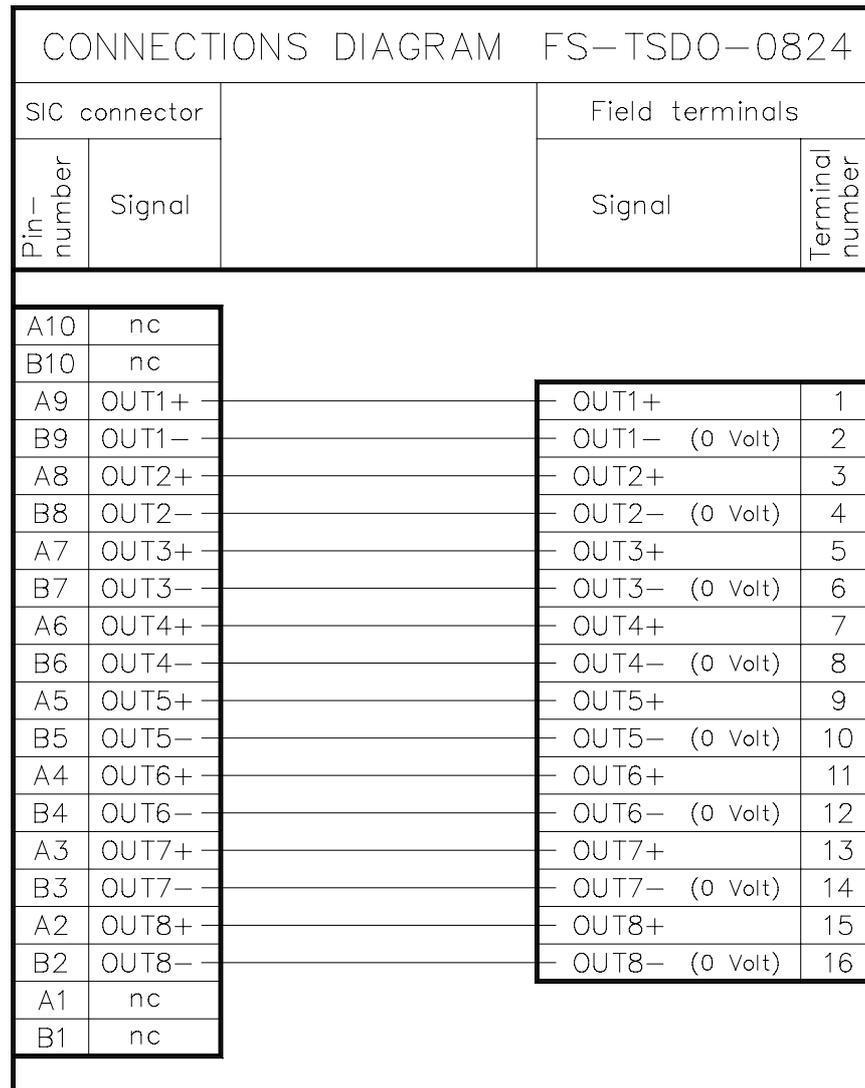
Figure 2 Connections diagram
