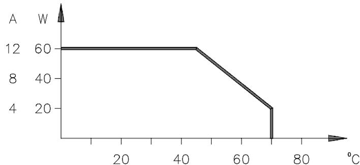
Figure 3 Derating curve (current and power vs. ambient temperature)
