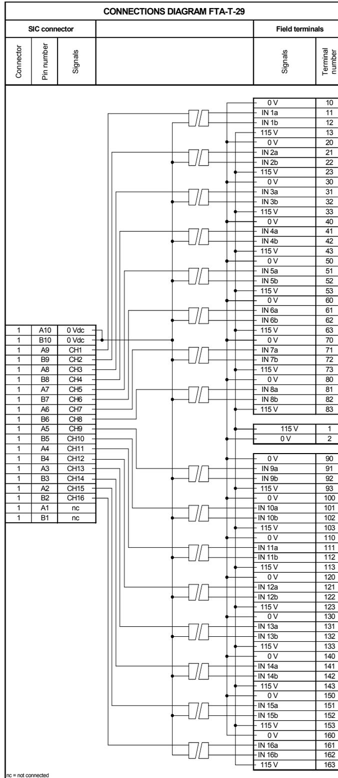
Figure 8 Connections diagram
