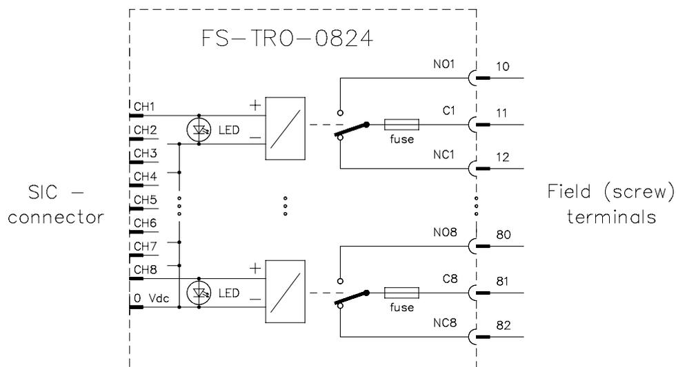
Figure 2 Schematic diagram
