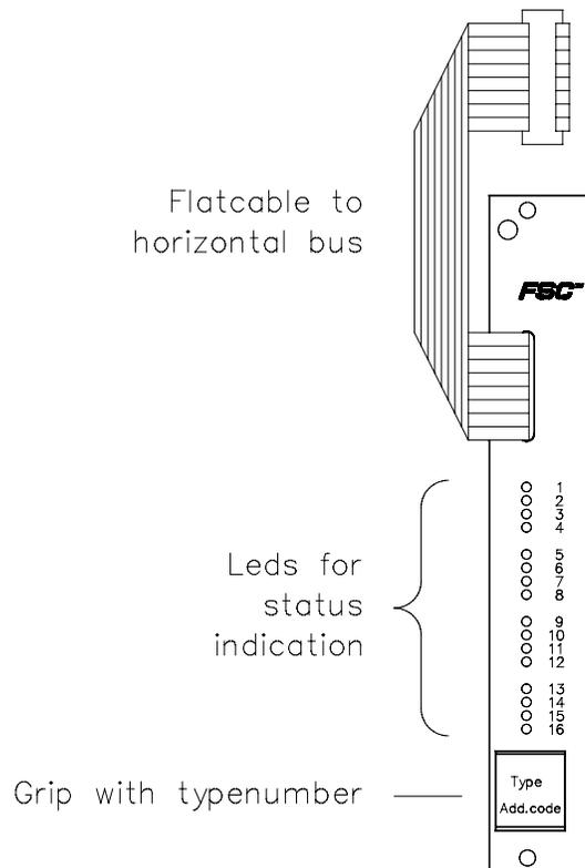
Figure 1 Front of a digital input module
