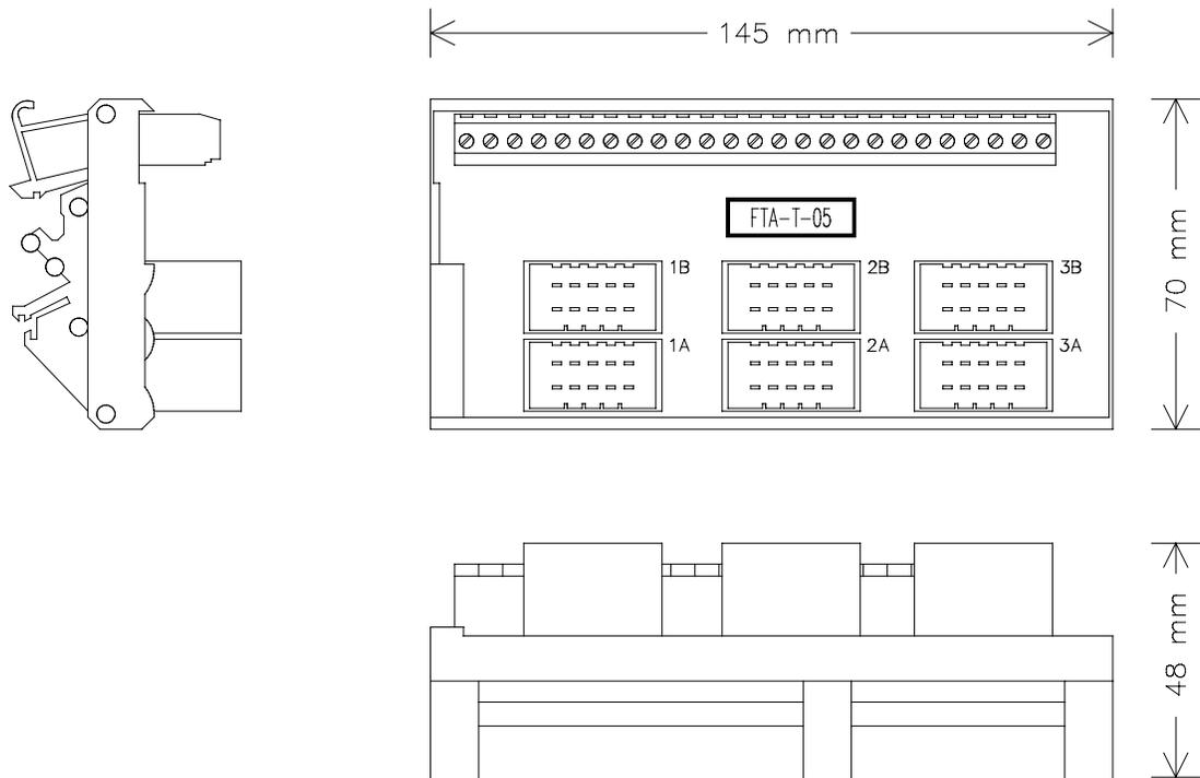
Figure 1 Mechanical layout
