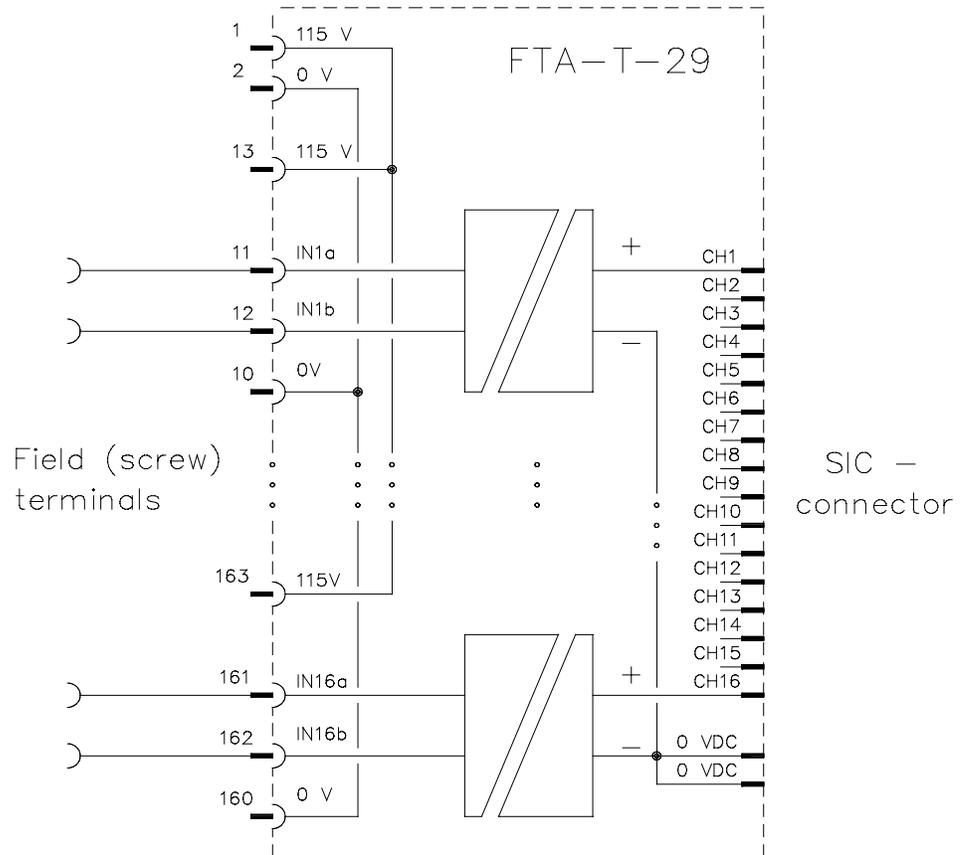
Figure 6 Schematic diagram for connecting active inputs.
