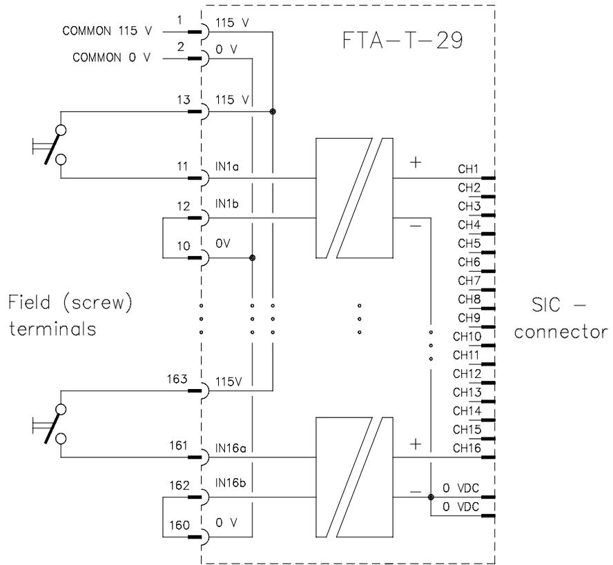
Figure 7 Schematic diagram for connecting passive inputs.
