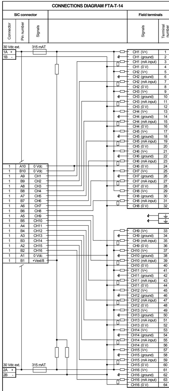
Figure 5 Connections diagram
