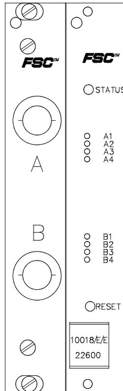
Figure 1 Front view of 10018/E/E module
