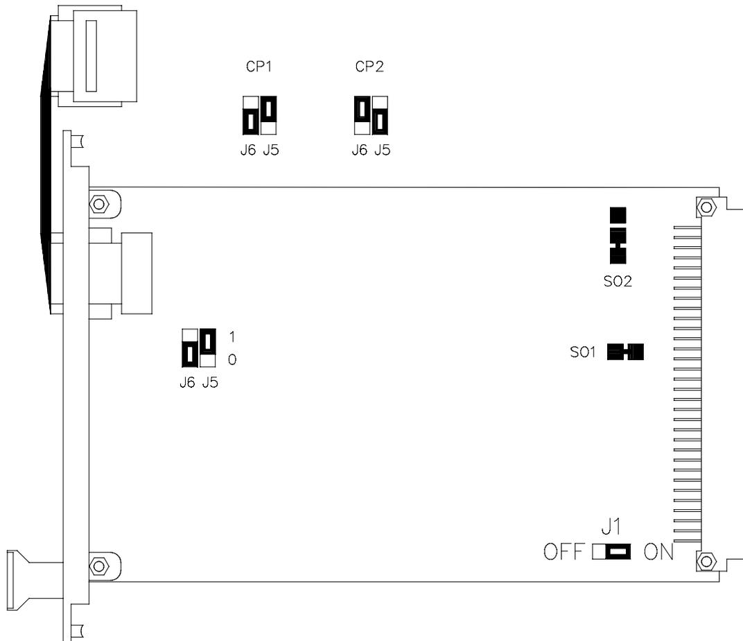
Figure 2 Jumper setting on 10007/1/1
