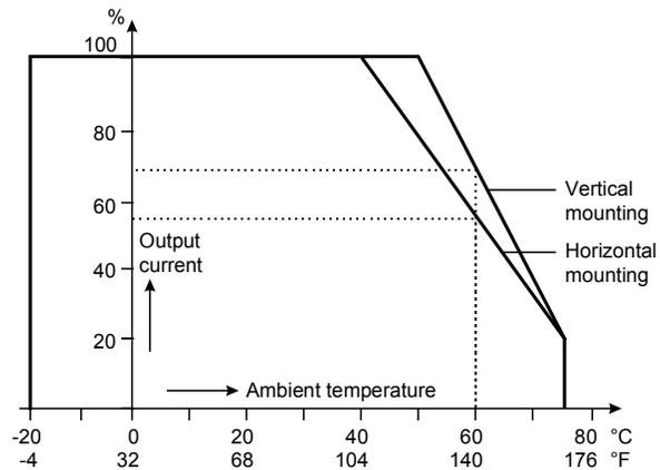
Figure 4 Derating curve
