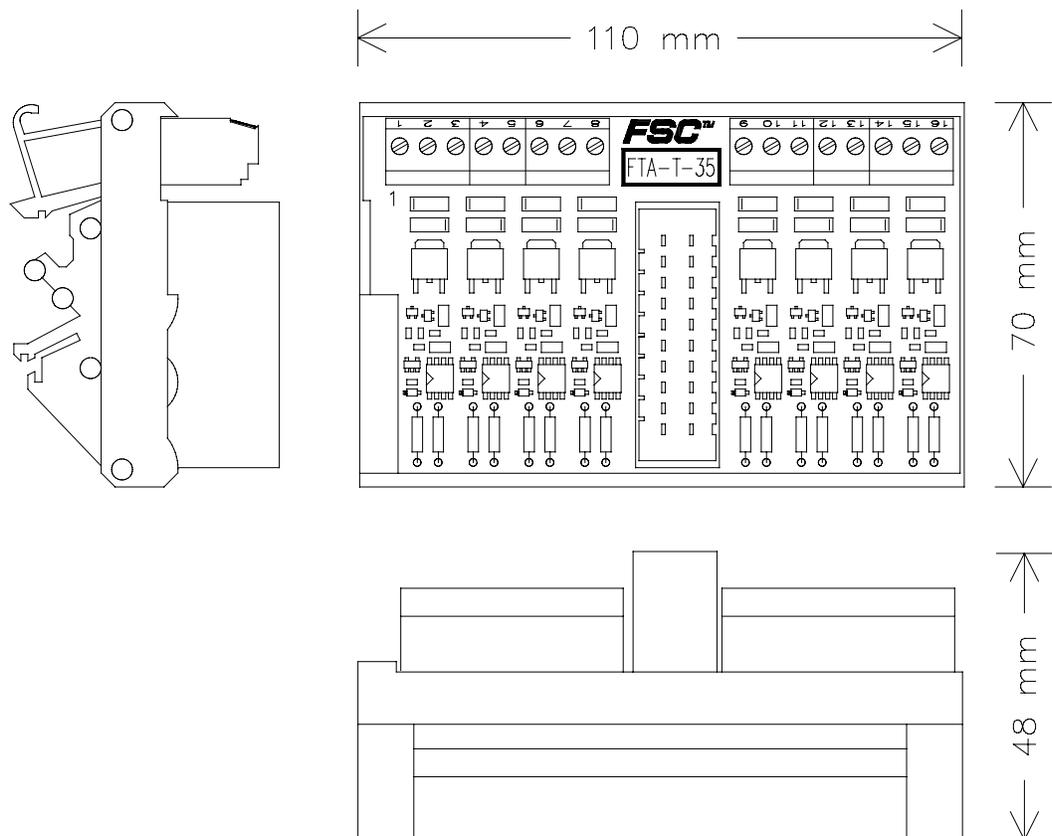
Figure 1 Mechanical layout
