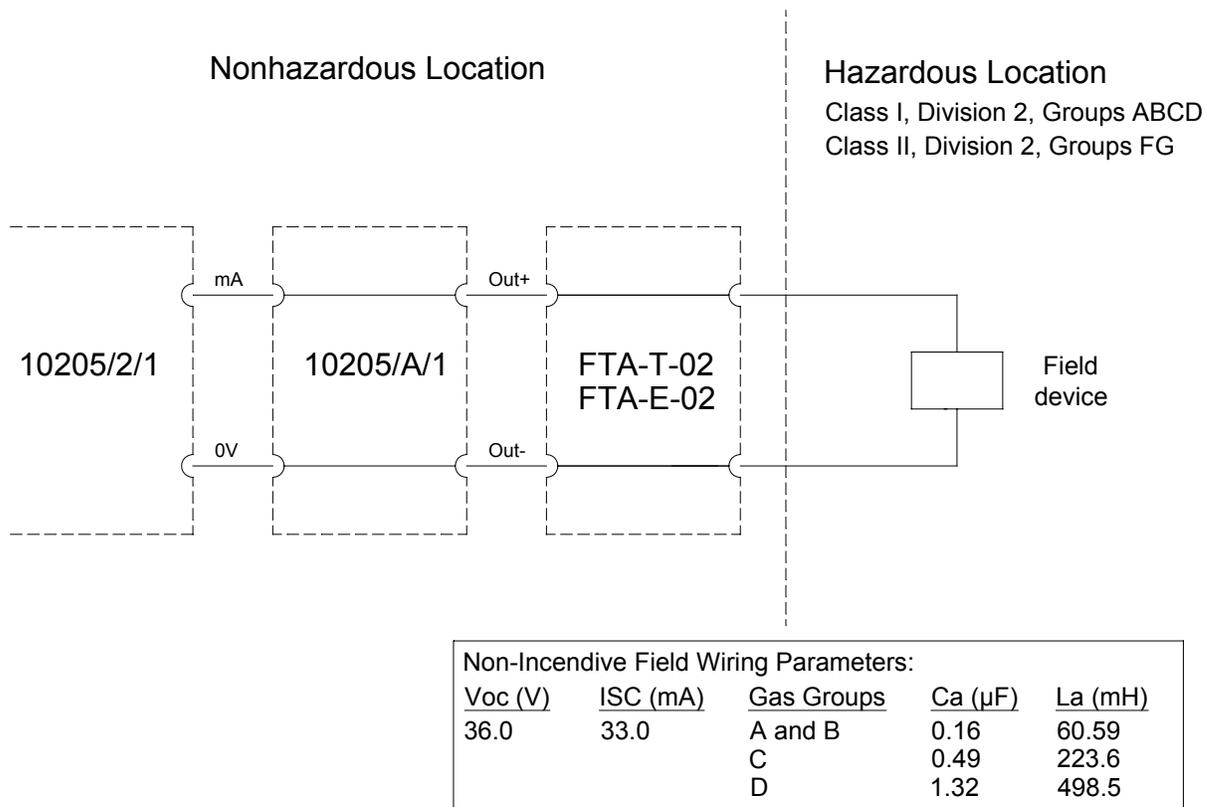
Figure 5 Connection of output in hazardous locations
