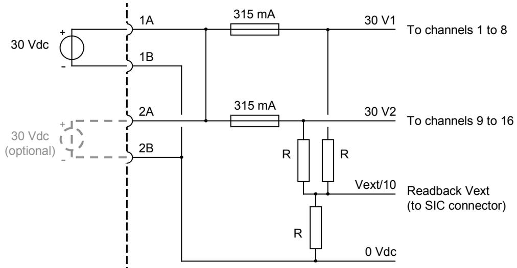
Figure 4 Schematic diagram for power distribution with monitoring
