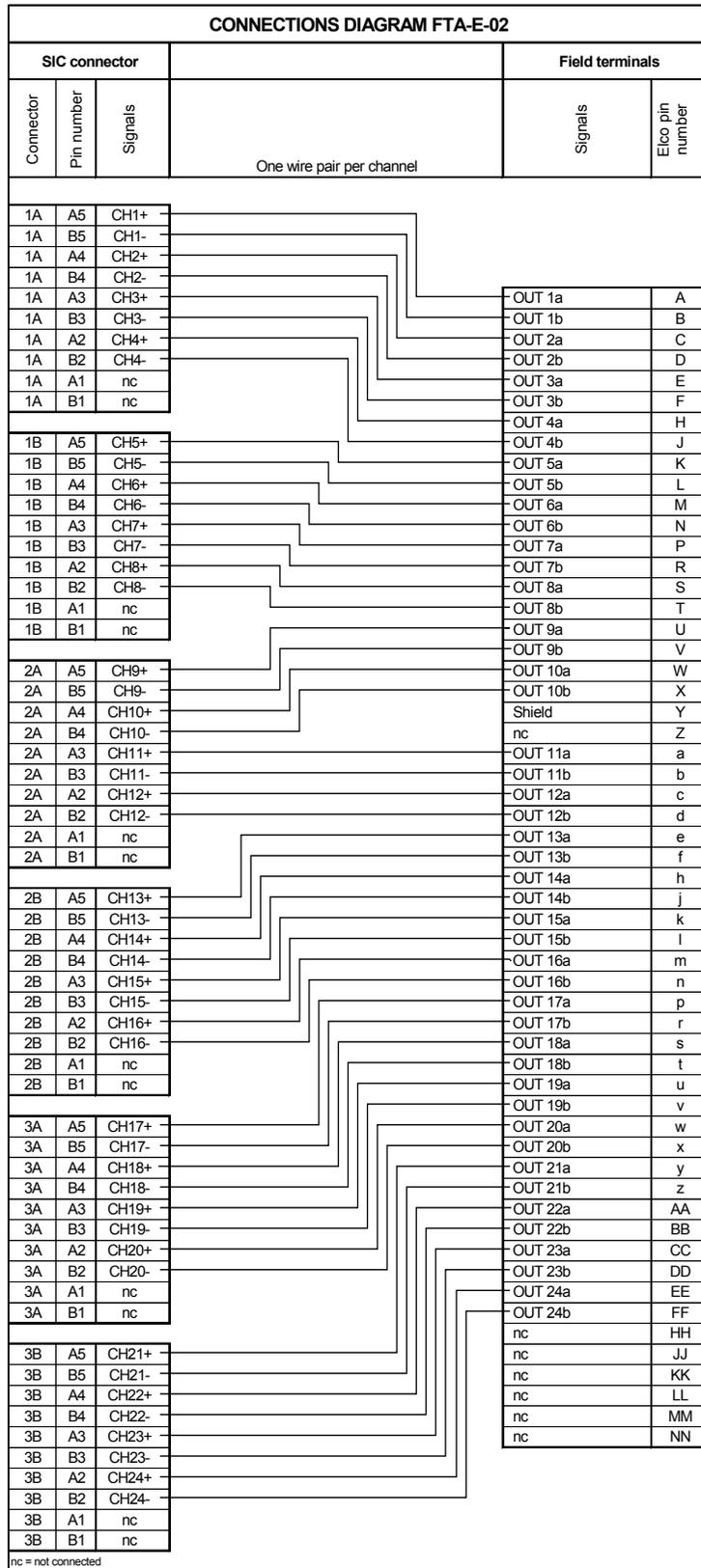
Figure 2 Connections diagram (one wire pair per channel)
