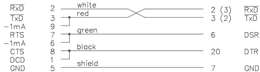
Figure 23 Connection between FSC system and printer:
