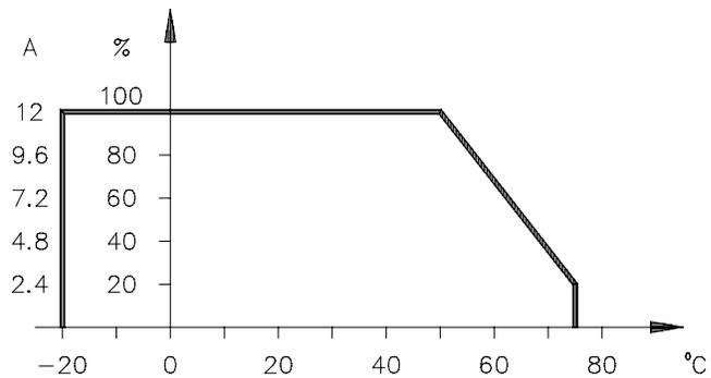
Figure 3 Derating curve (current & percentage of load vs. ambient temperature)
