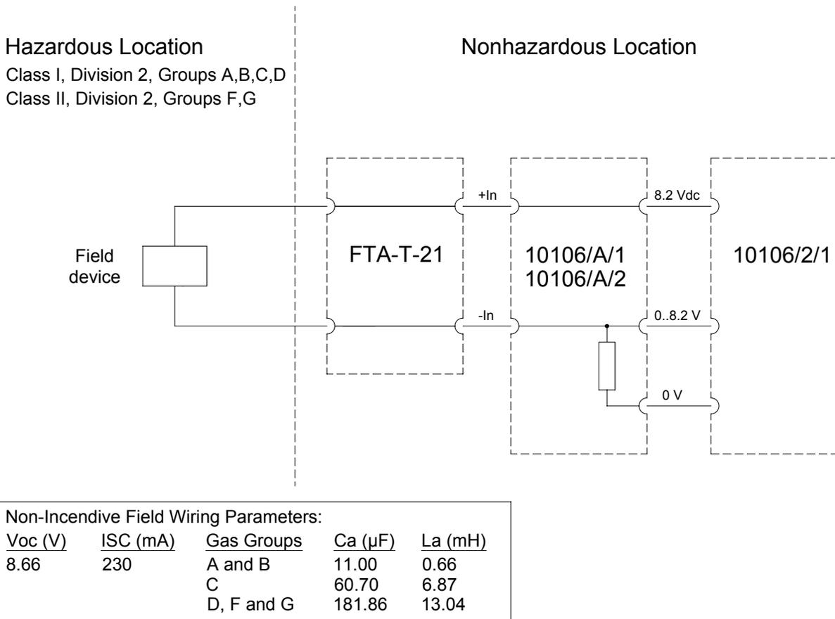
Figure 4 Connection of input in hazardous locations
