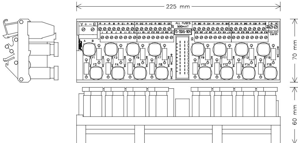
Figure 1 Mechanical layout
