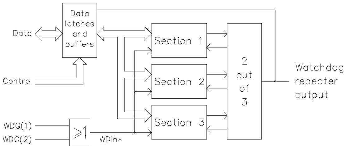
Figure 2 Block diagram for the watchdog repeater module
