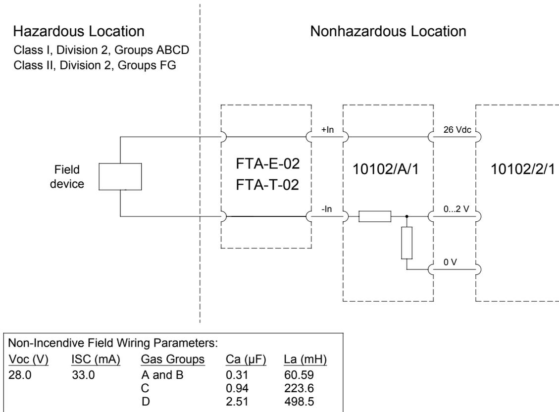
Figure 3 Connection of input in hazardous locations
