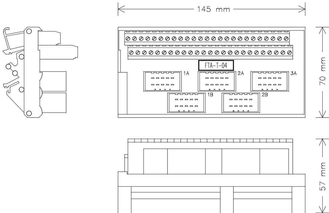
Figure 1 Mechanical layout
