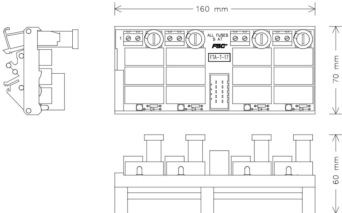
Figure 1 Mechanical layout
