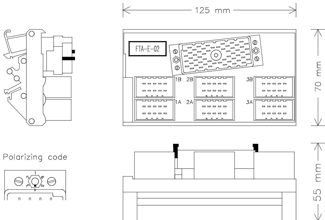
Figure 1 Mechanical layout
