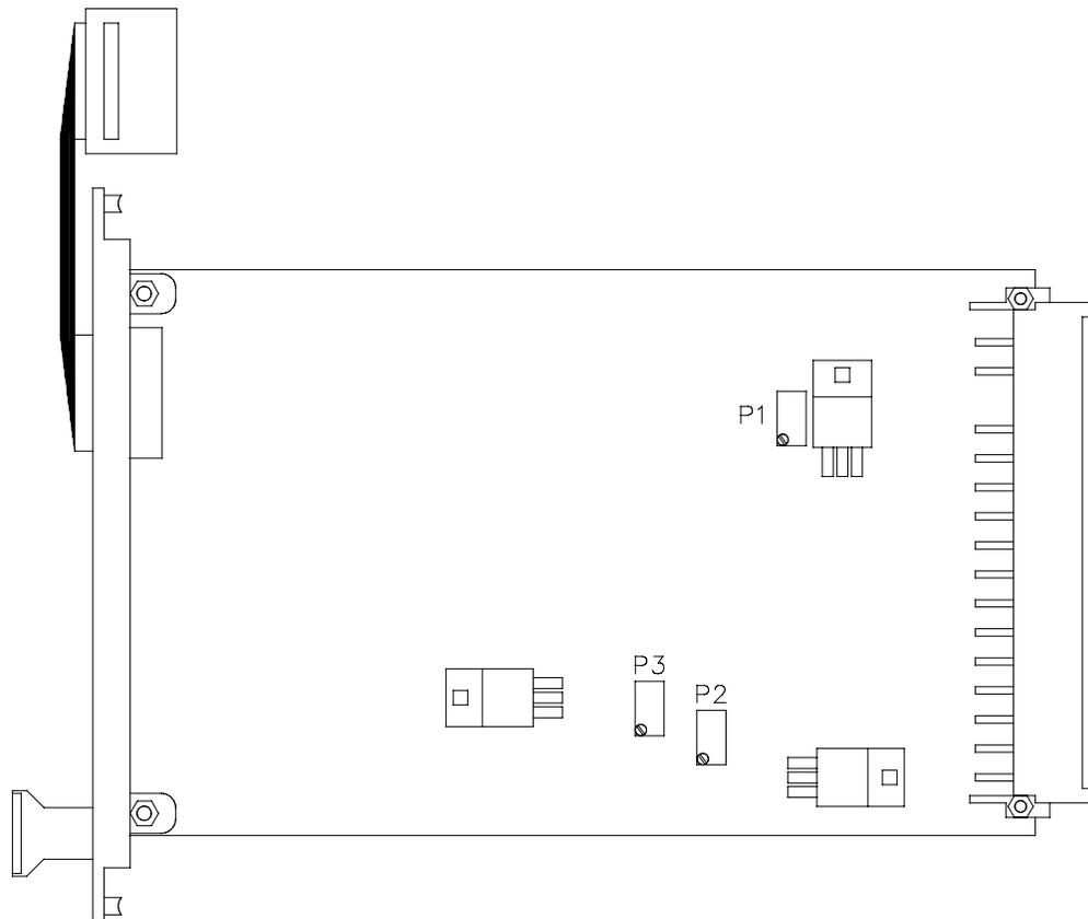
Figure 6 Location of potentiometers on 10205/2/1 module
