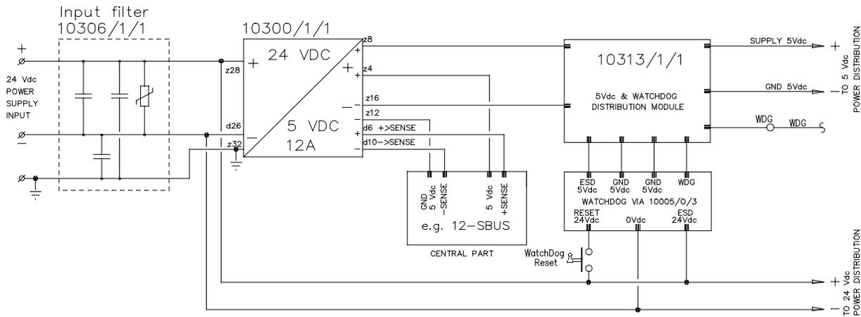
Figure 3 Connection details of 10005/O/3 for one Central Part
