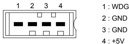
Figure 5 Pin connections of 'CP' and 'CP/CP-1' connector
