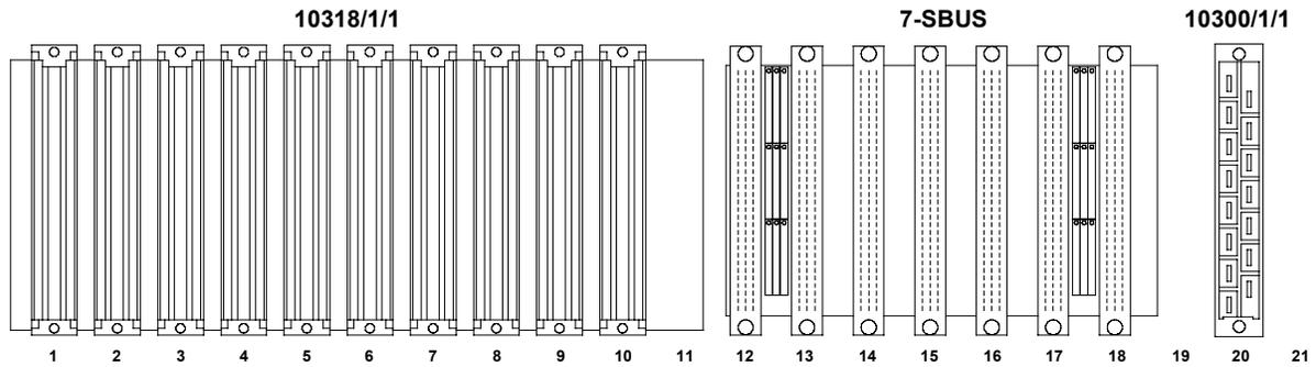
Figure 5 Front view of Central Part with I/O backplane and system bus
