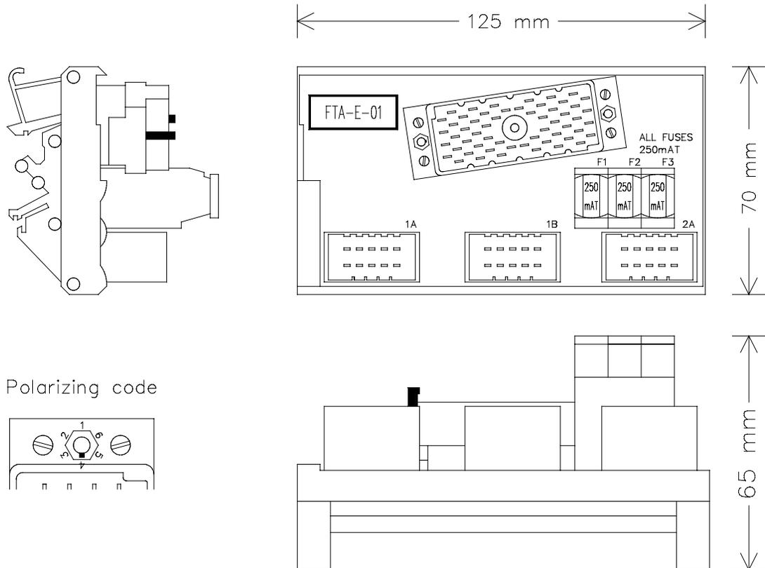
Figure 1 Mechanical layout
