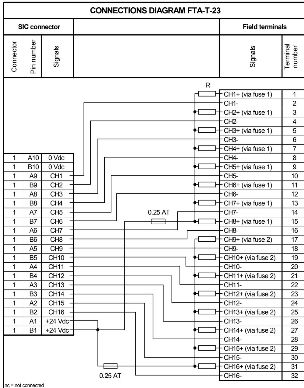
Figure 2 Connections diagram
