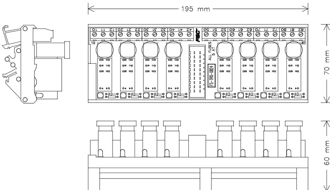
Figure 1 Mechanical layout
