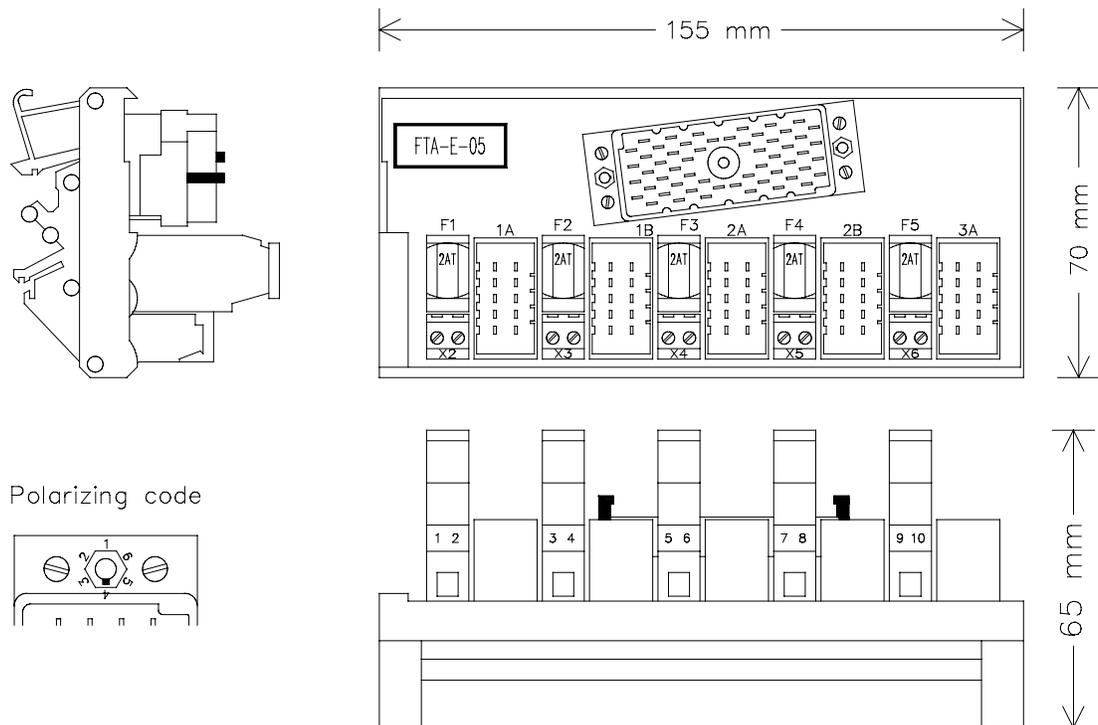
Figure 1 Mechanical layout
