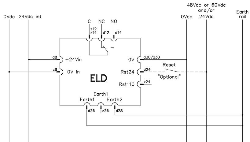
Figure 3 24 Vdc with 48 Vdc and/or 60 Vdc monitoring
