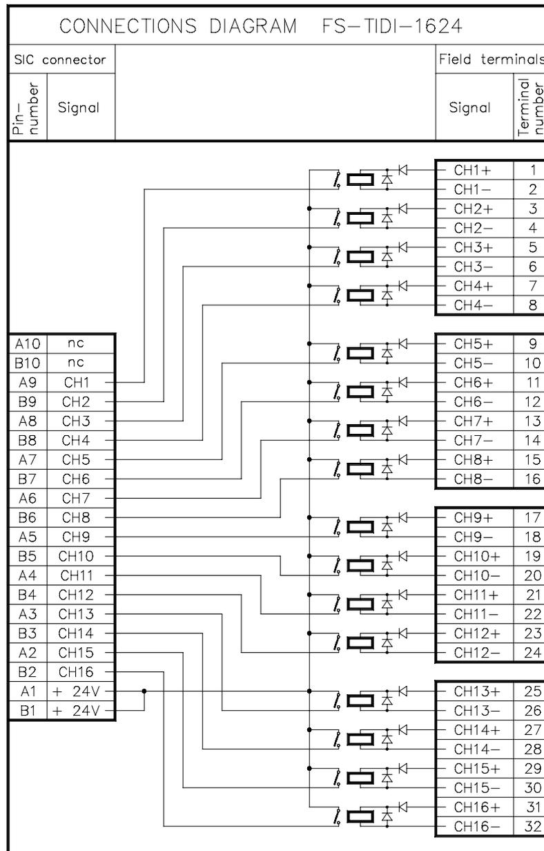
Figure 3 Connections diagram
