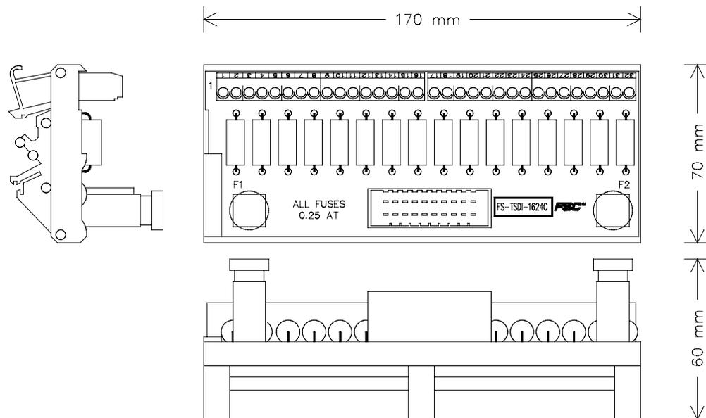
Figure 1 Mechanical layout
