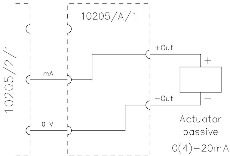
Figure 2 Schematic diagram of a 10205/A/1 module
