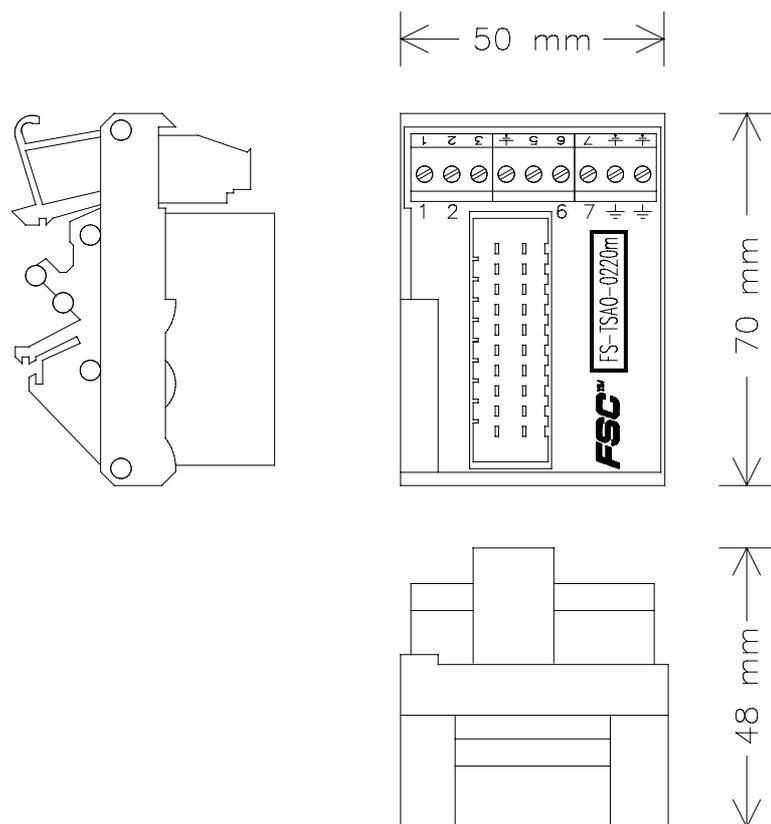
Figure 1 Mechanical layout
