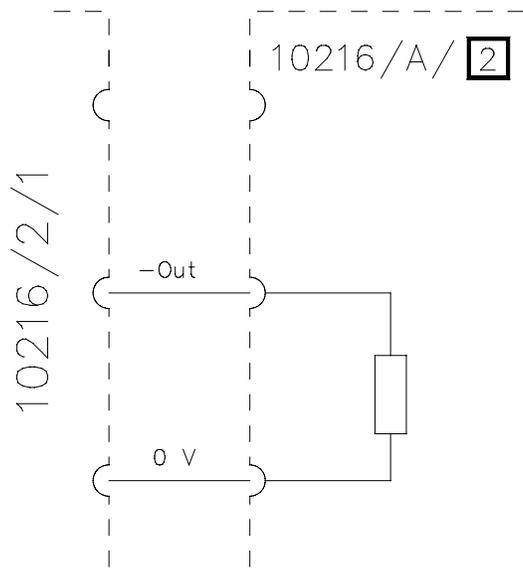
Figure 3 Schematic diagram of a 10216/A/2 module
