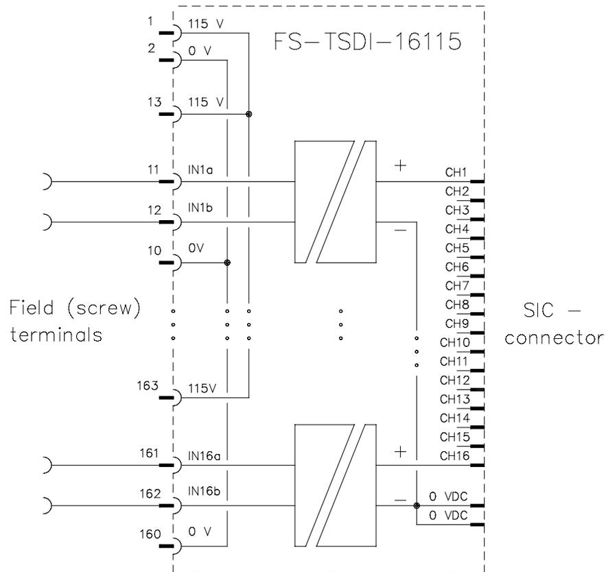
Figure 6 Schematic diagram for connecting active inputs.
