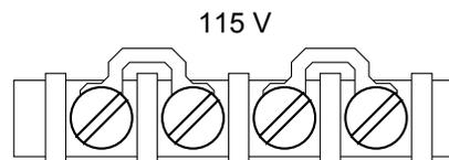
Figure 7 Selector block set at 115 V
