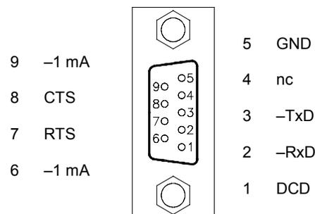
Figure 4 Front view of F-interface connector
