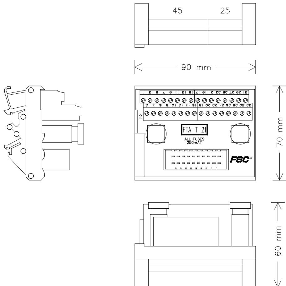
Figure 1 Mechanical layout
