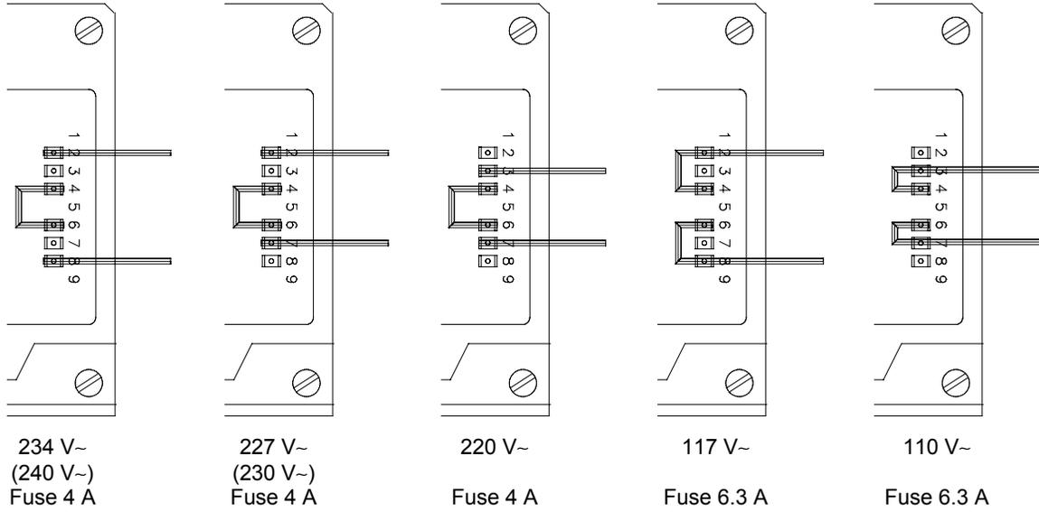
Figure 4 Transformer connections
