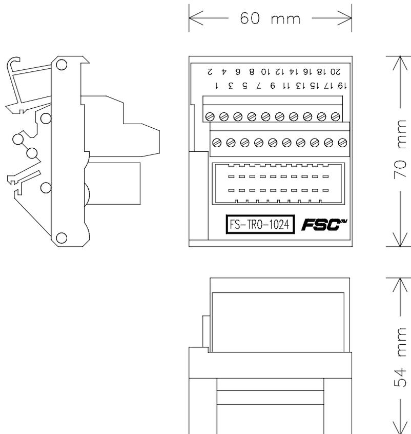
Figure 1 Mechanical layout
