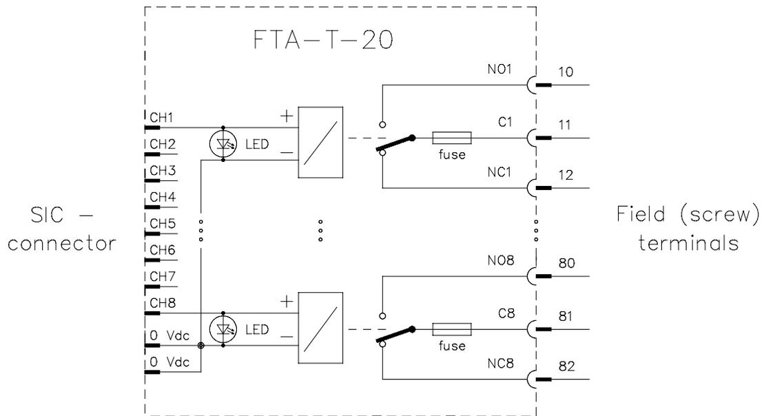
Figure 2 Schematic diagram
