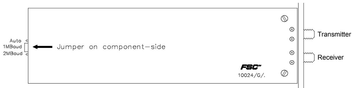
Figure 6 Jumper settings on G-interface
