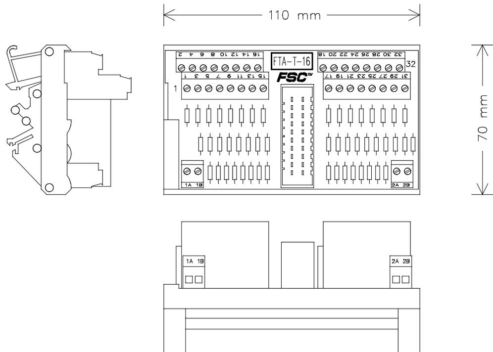
Figure 1 Mechanical layout
