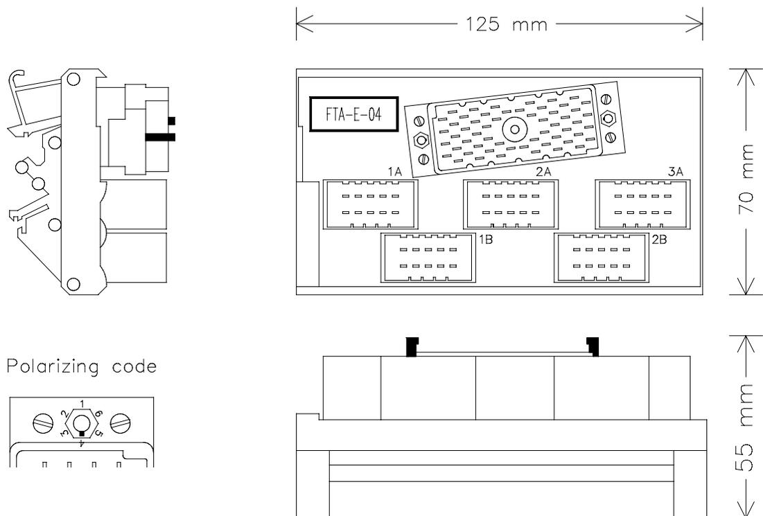
Figure 1 Mechanical layout
