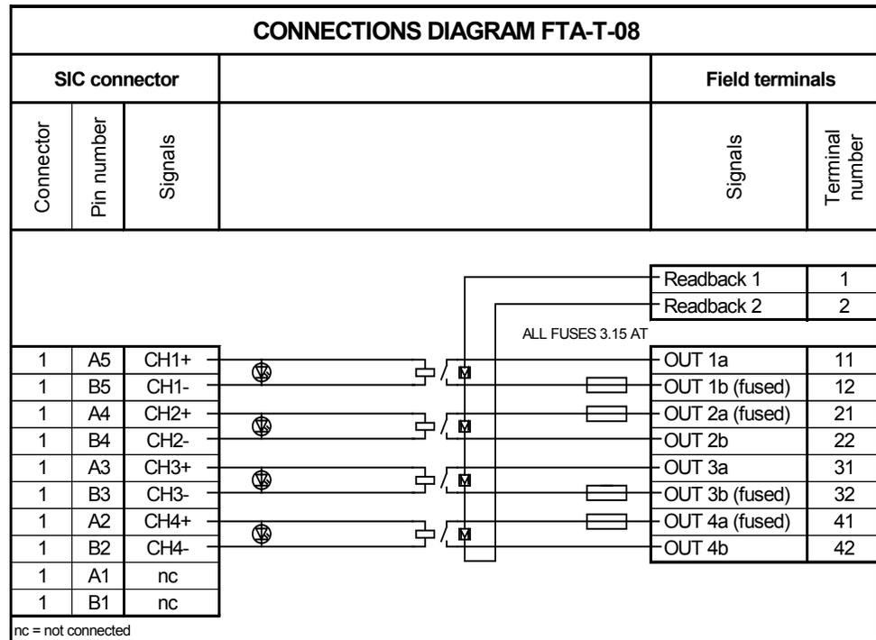
Figure 3 Connections diagram
