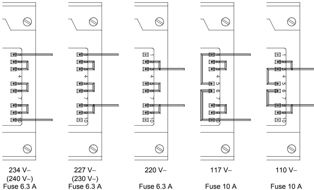
Figure 4 Transformer connections
