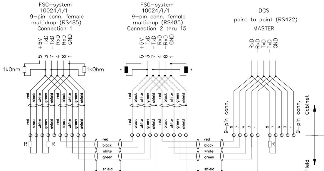
Figure 22 Connection between redundant FSC system and DCS
