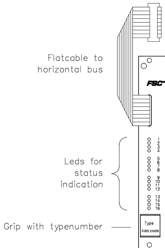
Figure 1 Front of a digital output module
