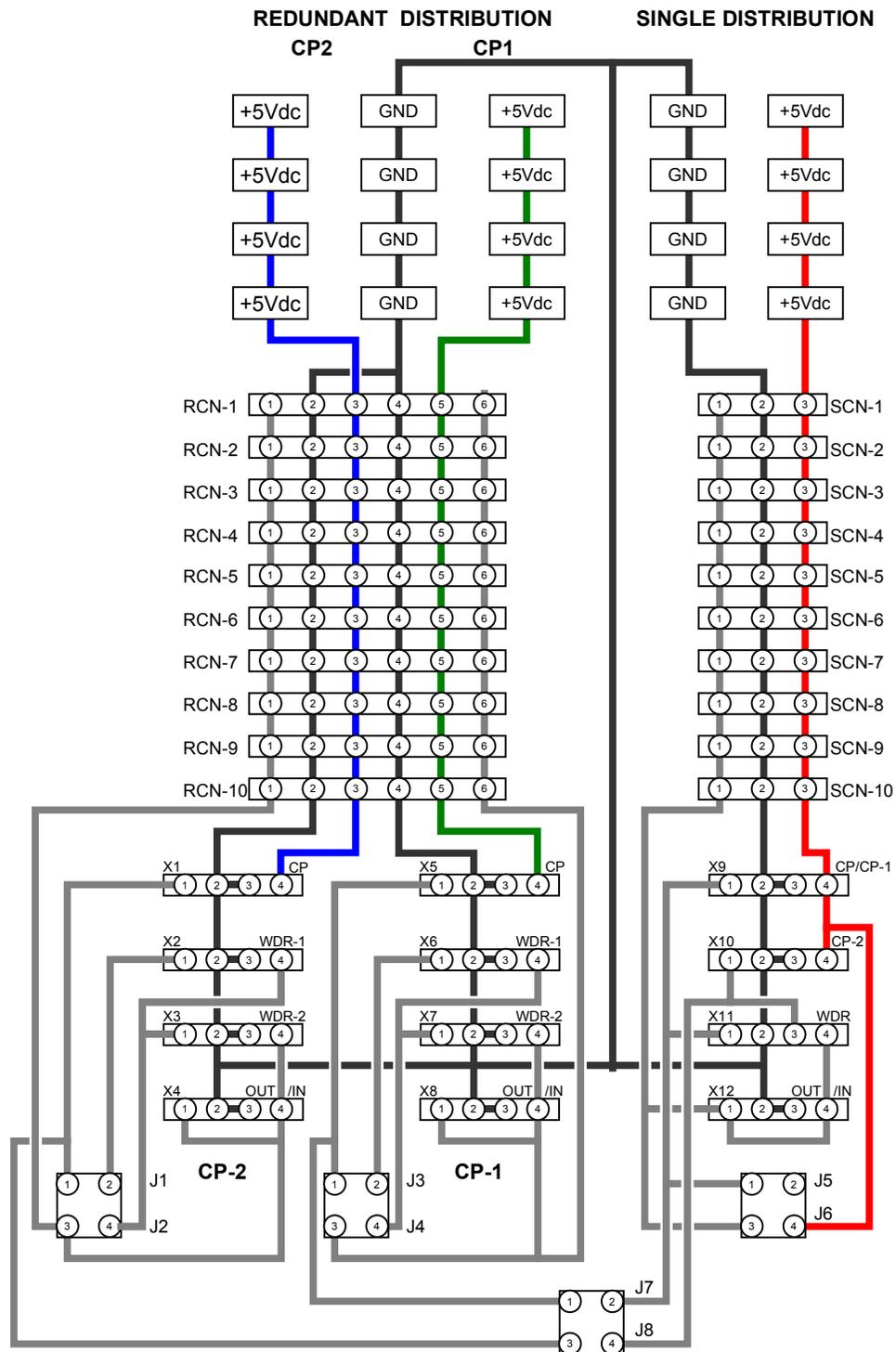
Figure 2 Connection diagram
