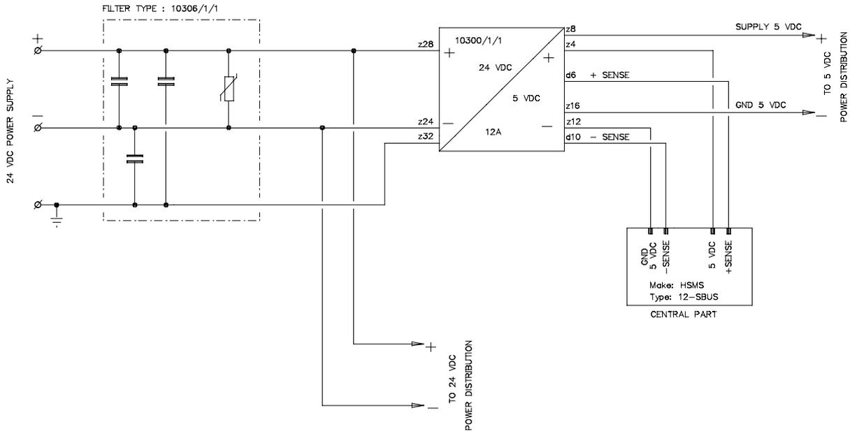
Figure 4 Wiring diagram
