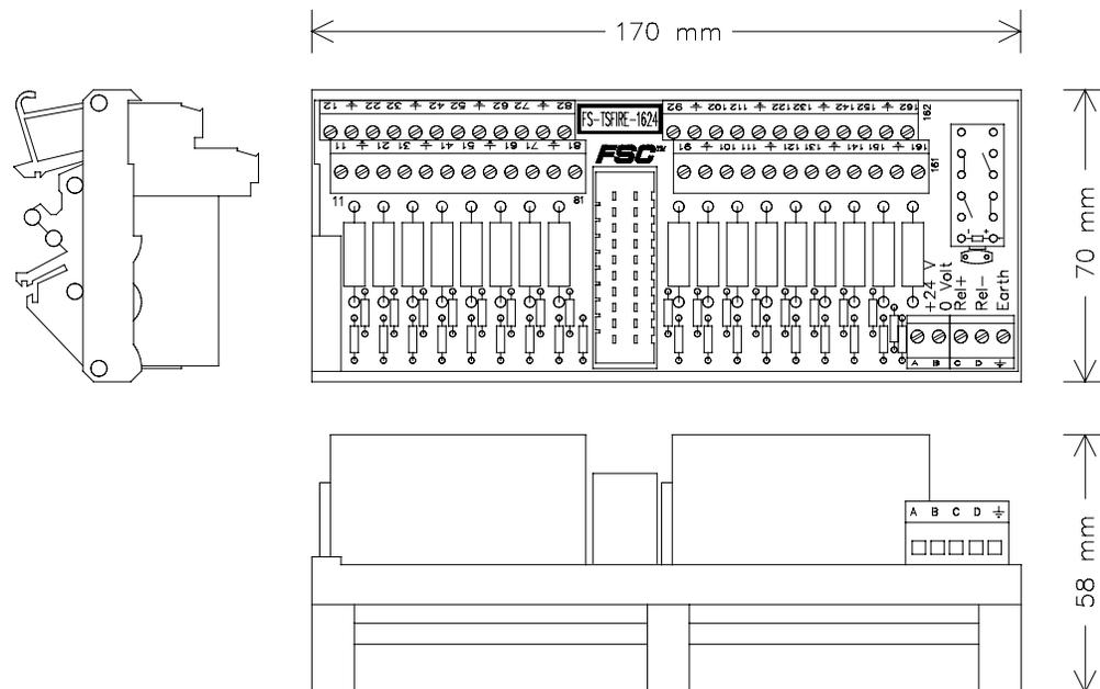
Figure 1 Mechanical layout
