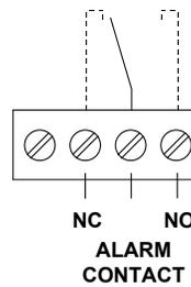
Figure 9 Relay contact alarm diagram
