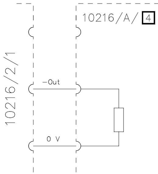
Figure 5 Schematic diagram of a 10216/A/4 module
