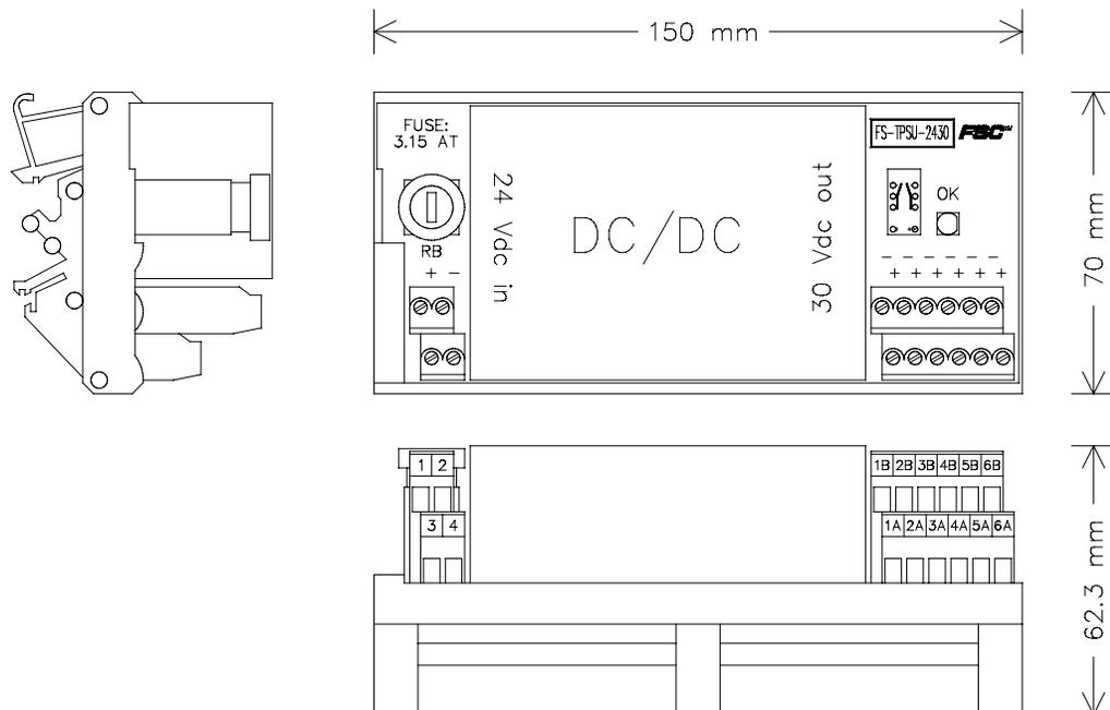
Figure 1 Mechanical layout
