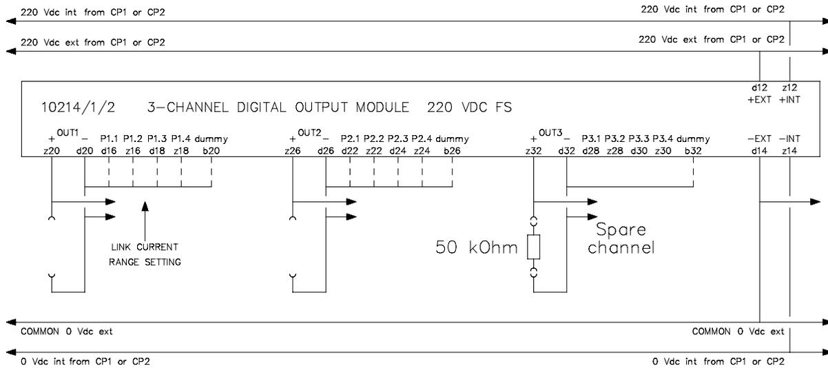
Figure 3 Connection example for redundant I/O configurations
