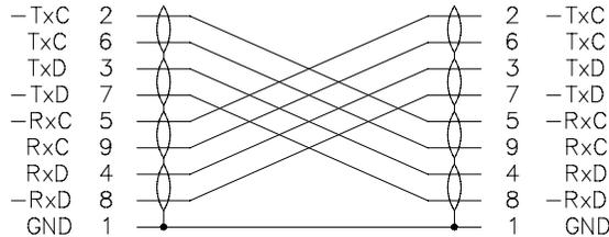
Figure 14 Connection between two Central Parts in redundant FSC configurations (using an H-interface)
