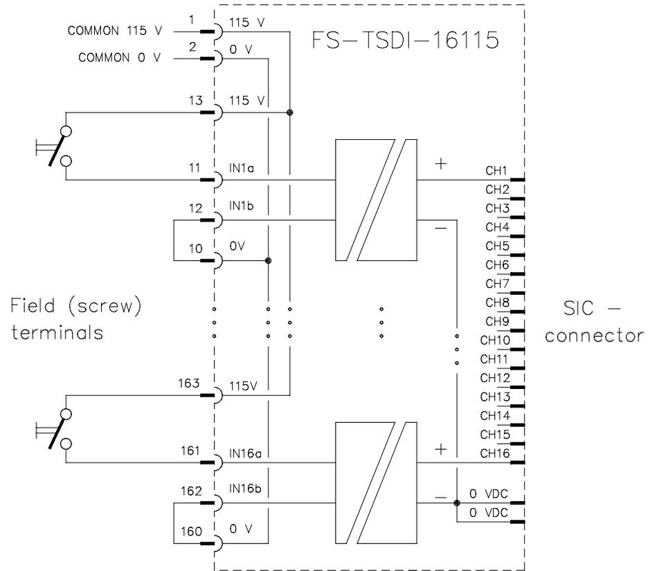
Figure 7 Schematic diagram for connecting passive inputs.
