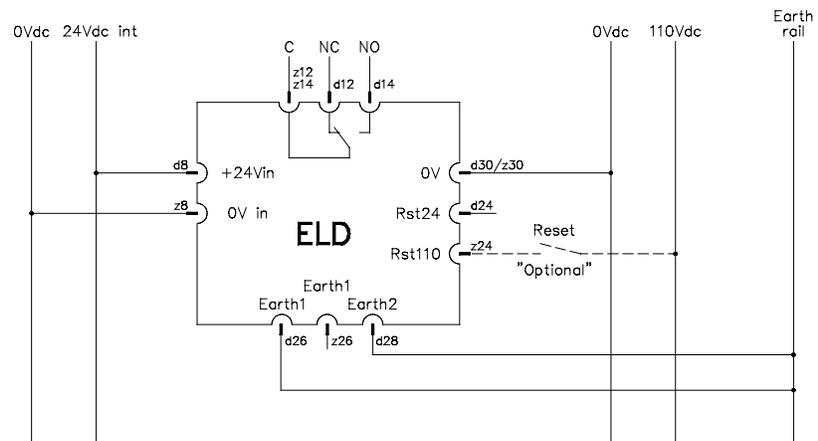
Figure 4 110 Vdc monitoring
