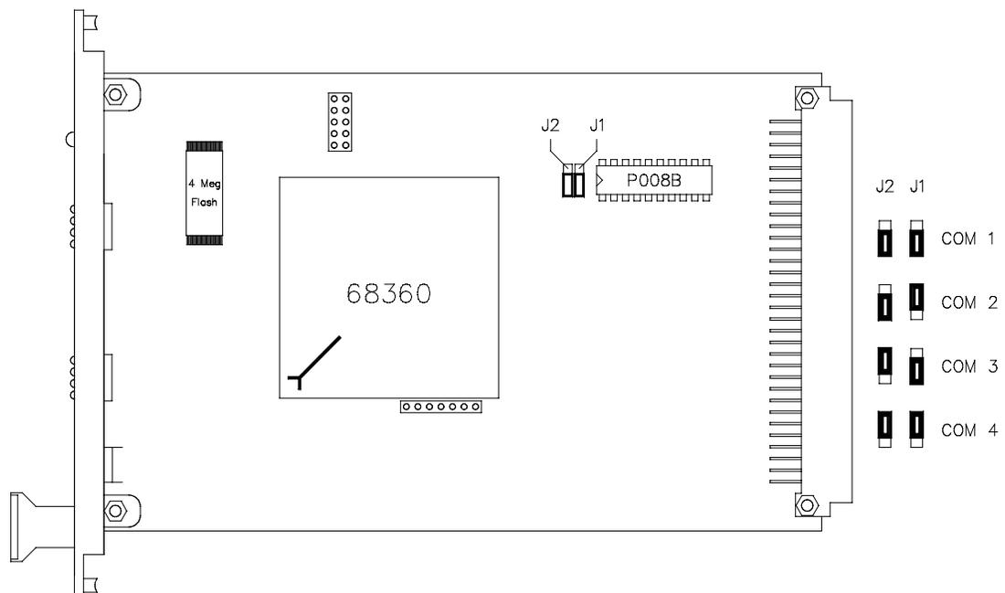
Figure 2 Jumper positions on 10018/E/1 & 10018/E/E main board
