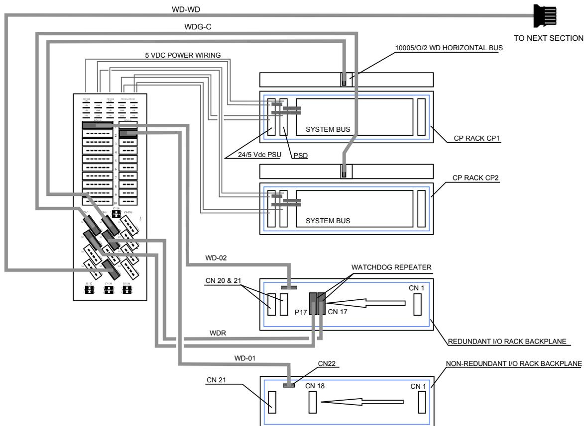
Figure 8 Concept diagram of 5 Vdc & watchdog distribution
