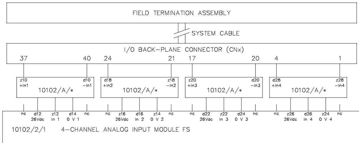
0V1, 0V2, 0V3 and 0V4 are galvanically connected on the pcb.
