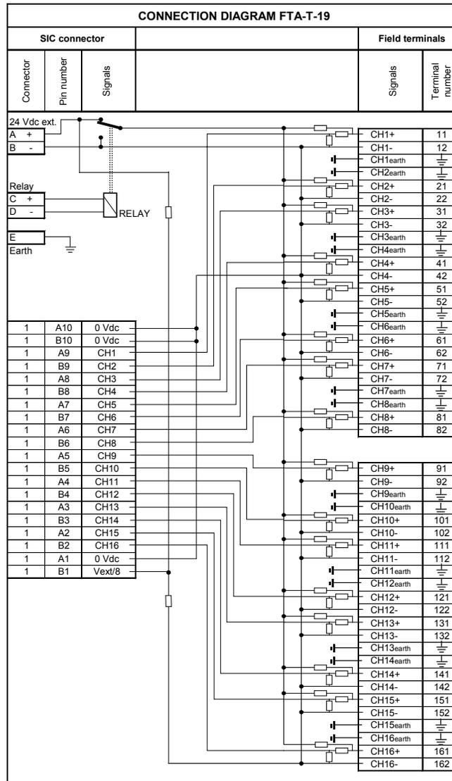
Figure 3 Connections diagram
