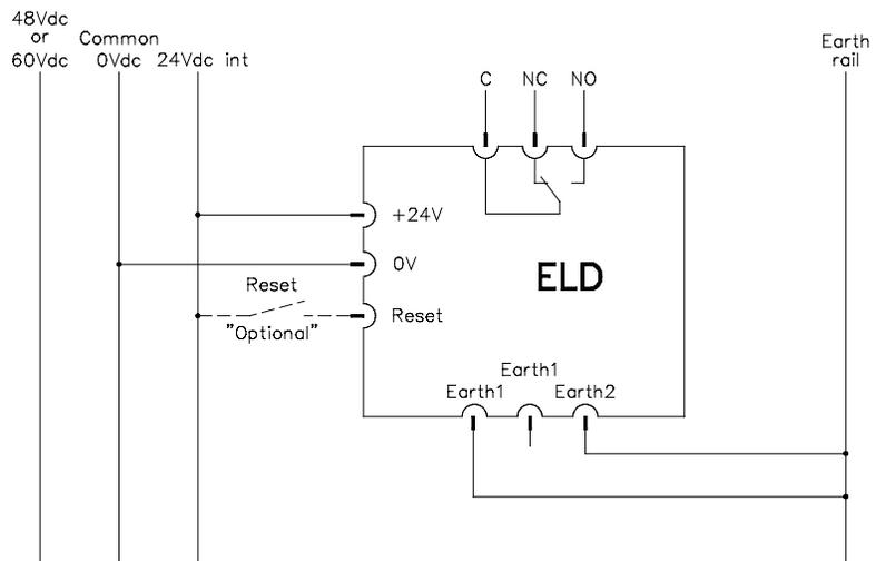
Figure 3 24 Vdc with 48 Vdc or 60 Vdc monitoring
