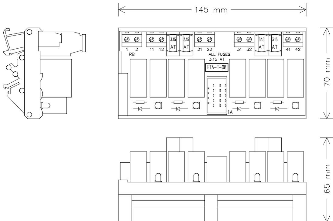
Figure 1 Mechanical layout
