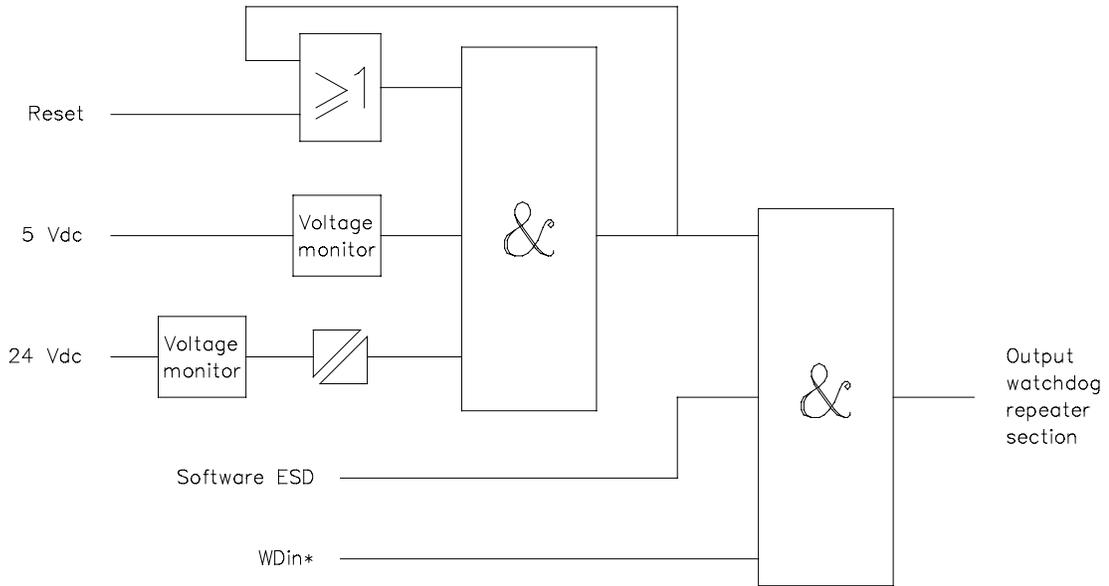
Figure 1 Logic diagram for a watchdog repeater section
