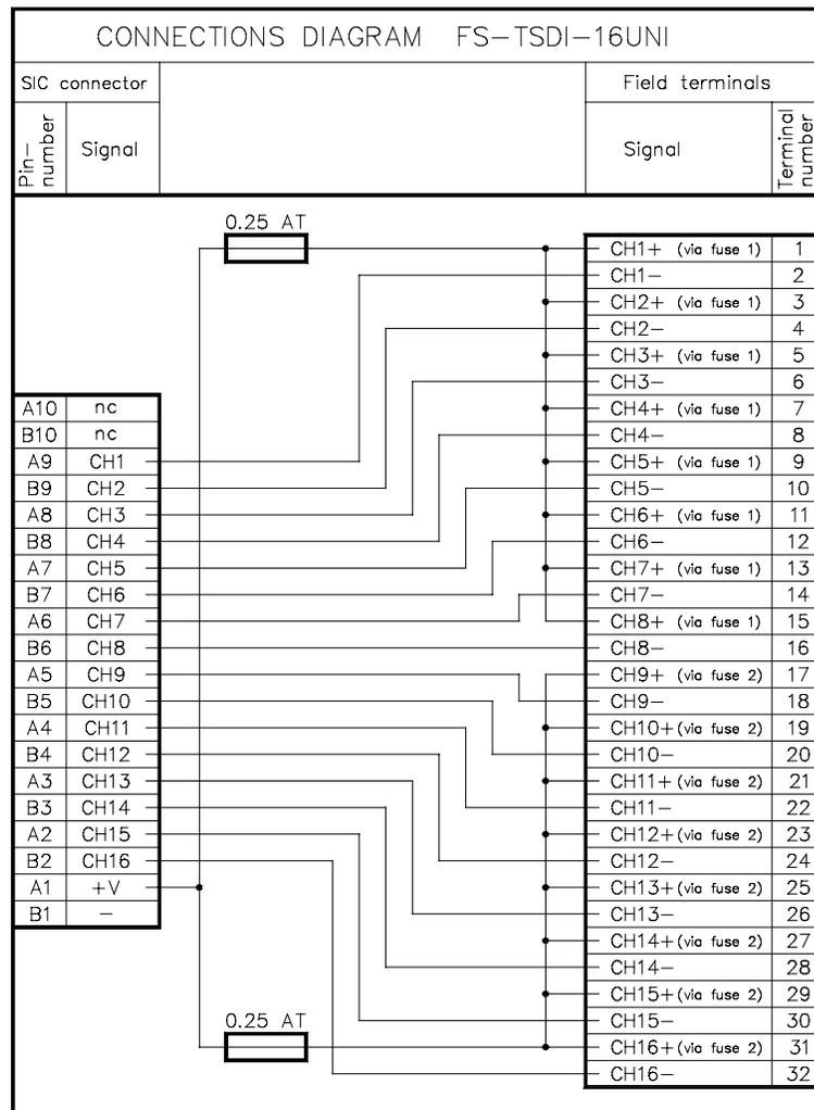
Figure 2 Connections diagram
