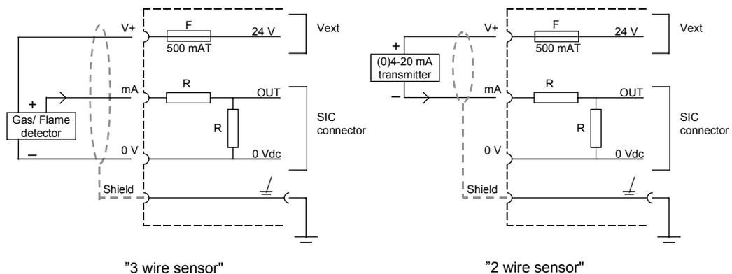
Figure 2 Schematic diagram for connecting a transmitter
