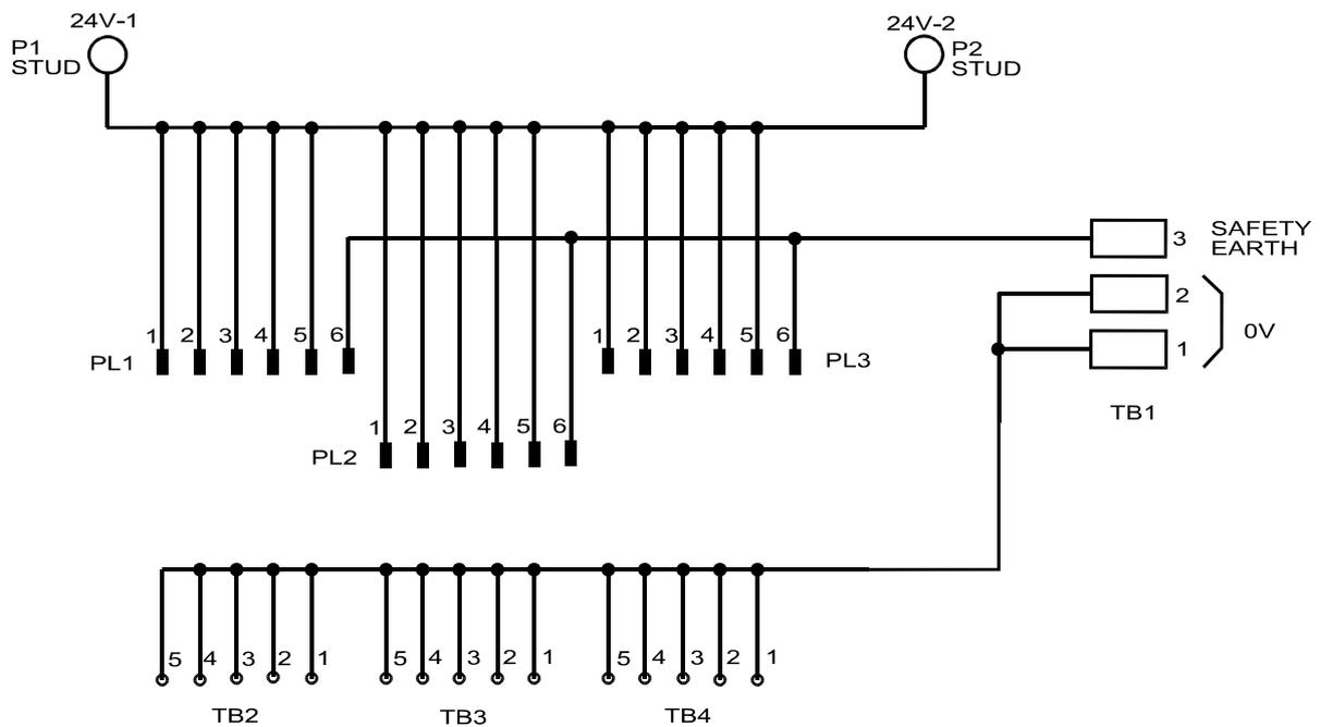
Figure 2 Trusted Output Power Distribution Unit – Wiring Diagram
