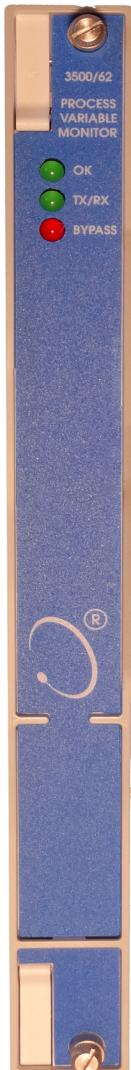
The Bently Nevada™ 3500/62 Process Variable Monitor is a 6-channel monitor for processing machine critical parameters that merit continuous monitoring, such as pressures, flows, temperatures, and levels. The monitor accepts +4 to +20 mA current inputs or any proportional voltage inputs between -10 Vdc and +10 Vdc. It conditions these signals and compares the conditioned signals to user-programmable alarm setpoints.
