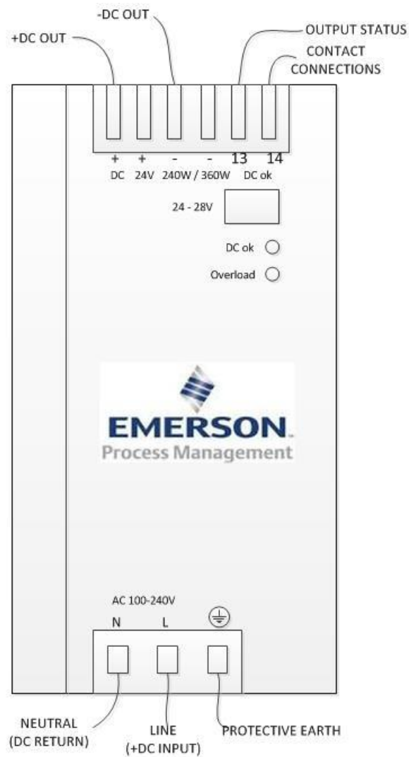
Figure 177: Power supply wiring illustration
